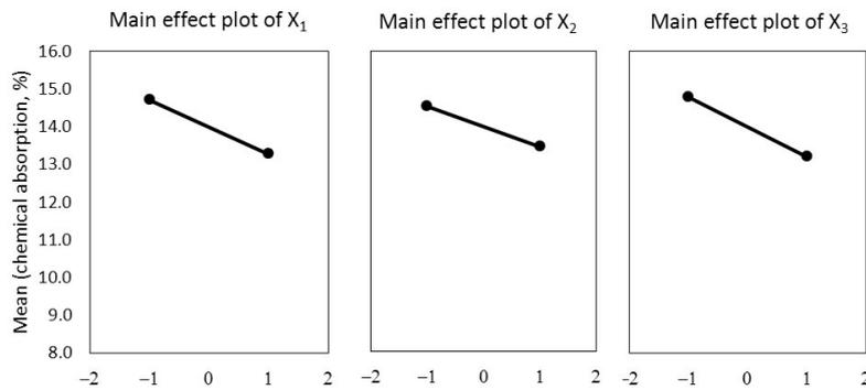
Fig. 3. Plots of the main effect of process input variables on chemical agent absorption.
