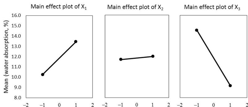
Fig. 1. Plots of the main effect of process input variables on water absorption.
