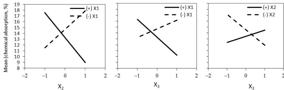
Fig. 4. Plots of the interaction effect of process input variables on chemical agent absorption.
