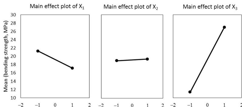
Fig. 5. Plots of the main effect of process input variables on bending strength.
