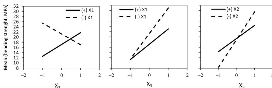
Fig. 6. Plots of the interaction effect of process input variables on bending strength.
