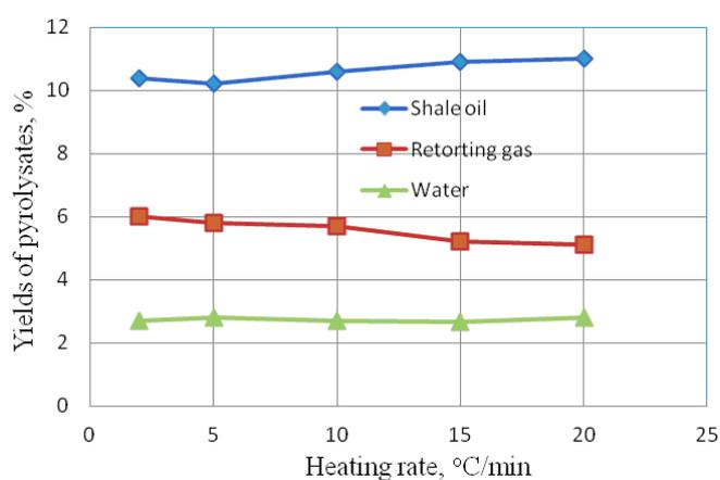
Fig. 6. Influence of heating rate on pyrolysates yield.
