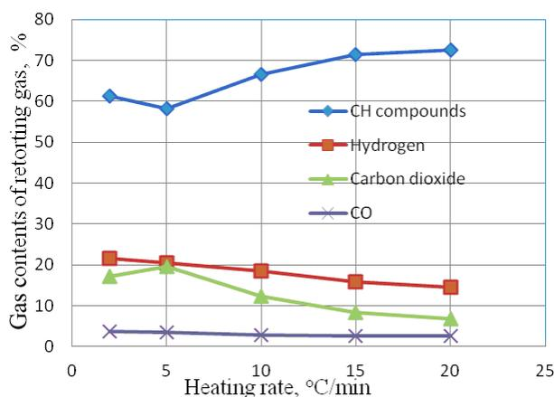
Fig. 7. Influence of heating rate on the composition of retorting gas.
