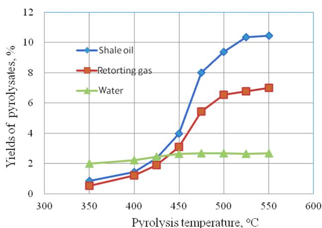
Fig. 2. Yields of pyrolysates at different pyrolysis temperatures.
