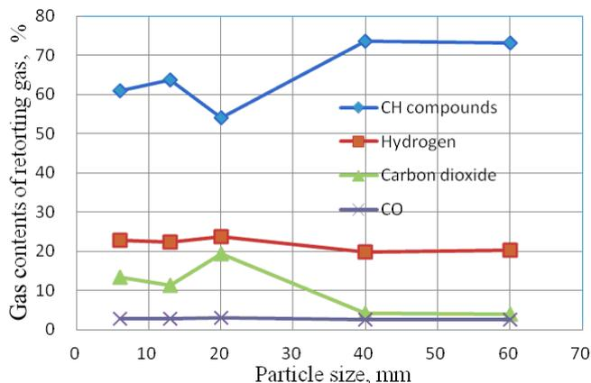
Fig. 9. Influence of particle size on the composition of retorting gas.
