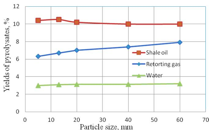
Fig. 8. Influence of particle size on pyrolysates yield.
