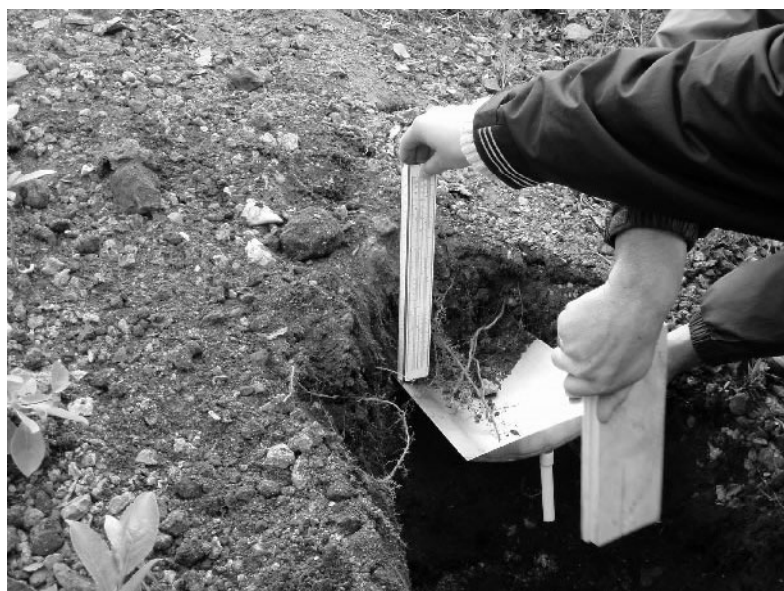
Fig. Installation of a sampler at the closed site of the spent shale deposit.
