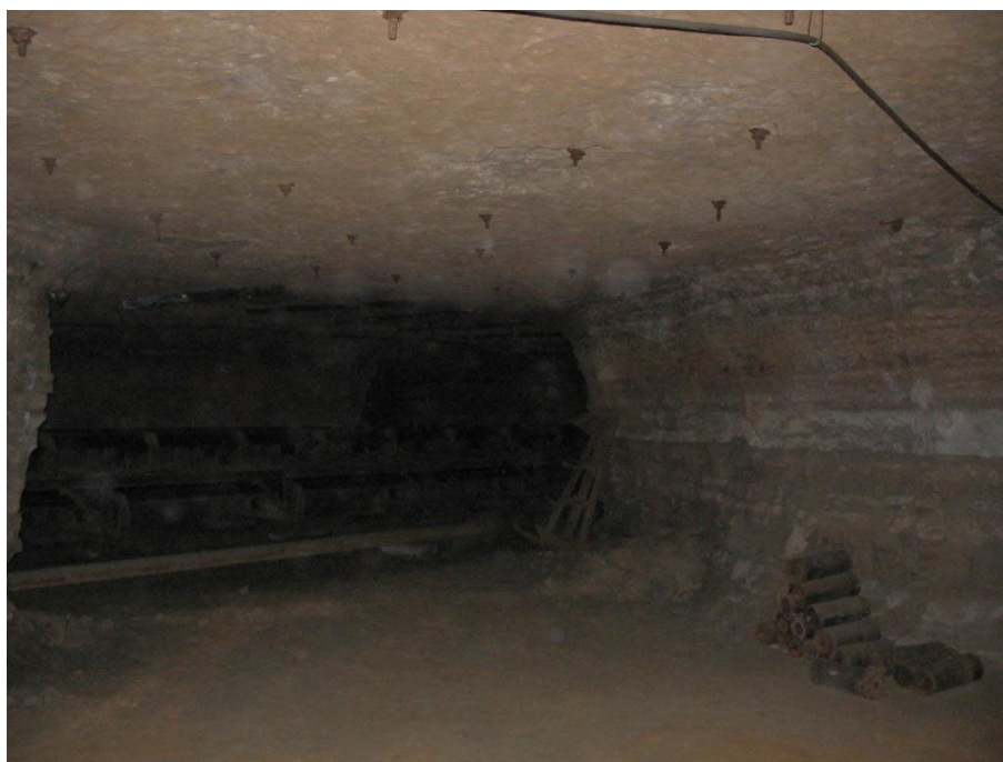
Fig. 6. Room and pillar mining leaves underground free space (Estonia mine) [16].
