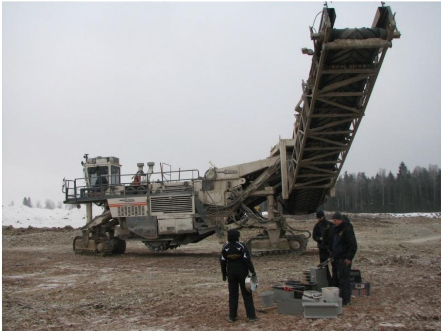
Fig. 12. Mechanical sieving of crushed material by Wirtgen 2500 SM in field works.
