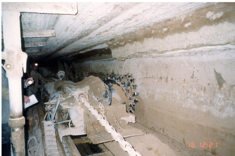
Fig. 2. Partial seam longwall mining of oil shale.
