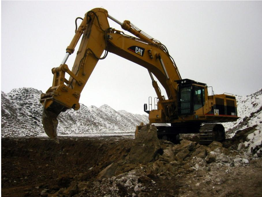
Fig. 7. Breaking oil shale seam with hydraulic excavator.
