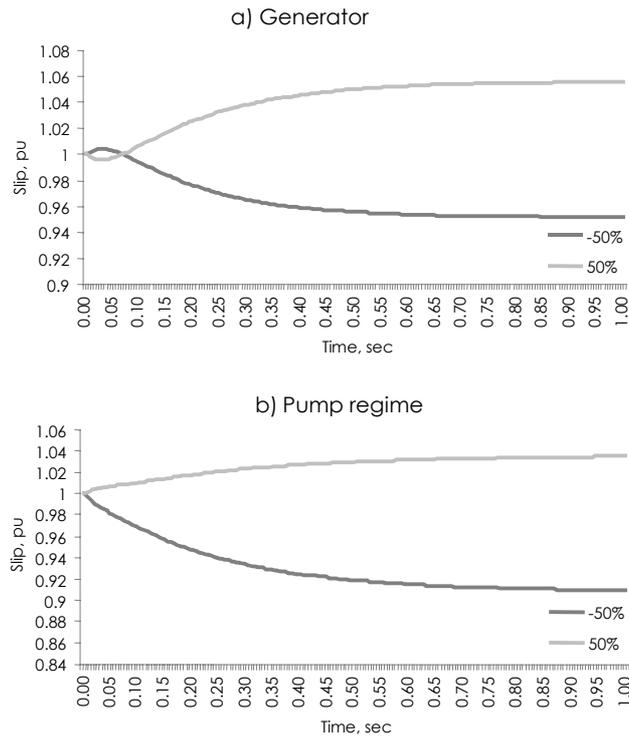
Fig. 5. Graphics of the time dependence of rotor slip.
