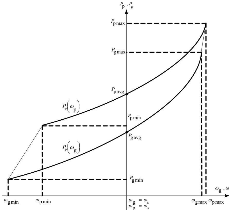
Fig. 2. Dependence of the hydraulic turbine power on the angular frequency.
