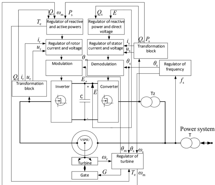
Fig. 3. Structure diagram of an exciter control system.
