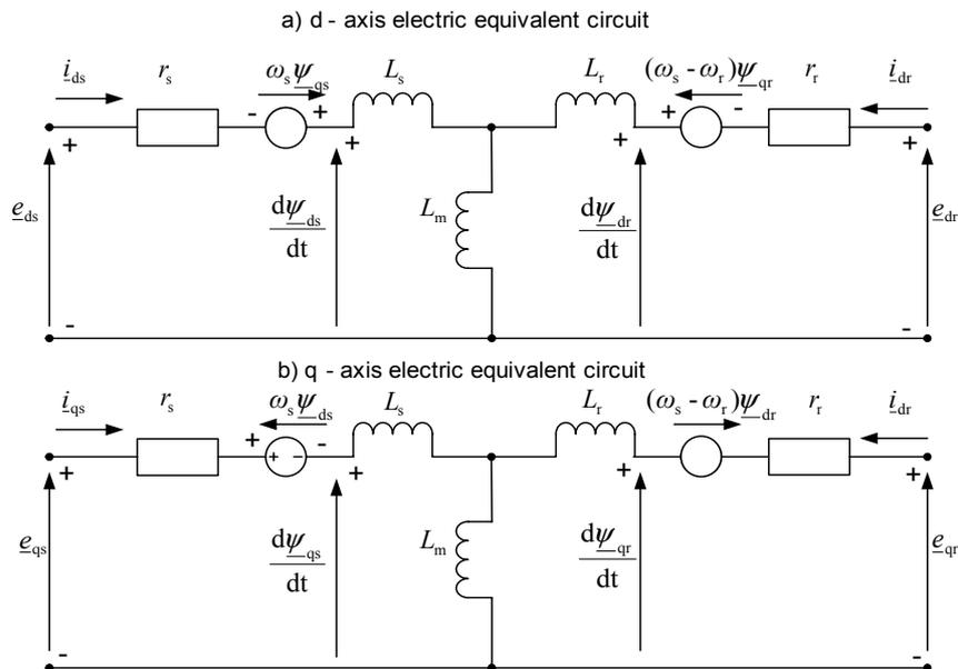
Fig. 1. Equivalent diagrams of VSPSU corresponding to d and q parameters.
