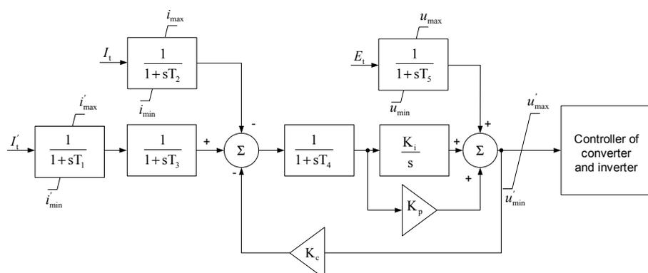
Fig. 4. Mathematical model of a simplified exciter control system.
