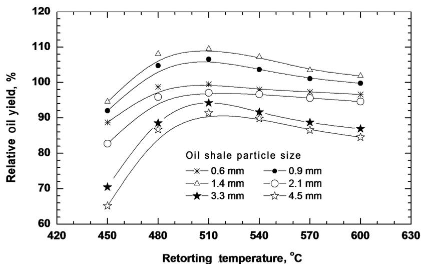
Fig. 2. Change of percentage relative oil yield with retorting temperature at different shale particle sizes (shale hold time = 40 min).
