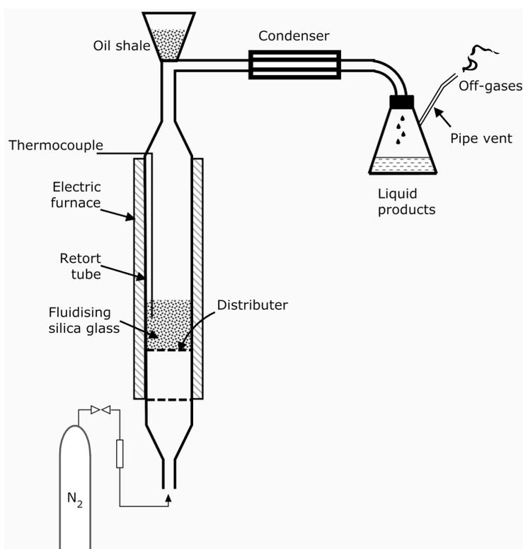
Fig. 1. Schematic diagram of the batch-loaded fluidized-bed reactor.
