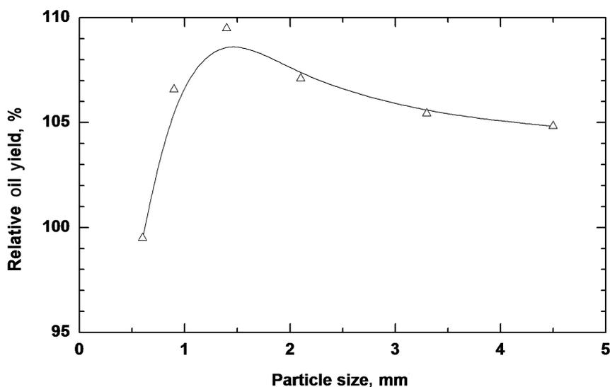
Fig. 4. Change of percentage relative oil yield with shale particle size at optimum retorting temperature of 510 °C (shale hold time 40 min).
