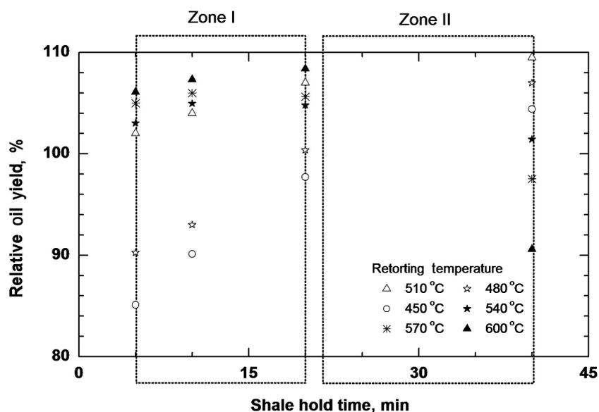
Fig. 5. Change of percentage relative oil yield with shale hold time at different retorting temperatures (shale particle size 1.4 mm).
