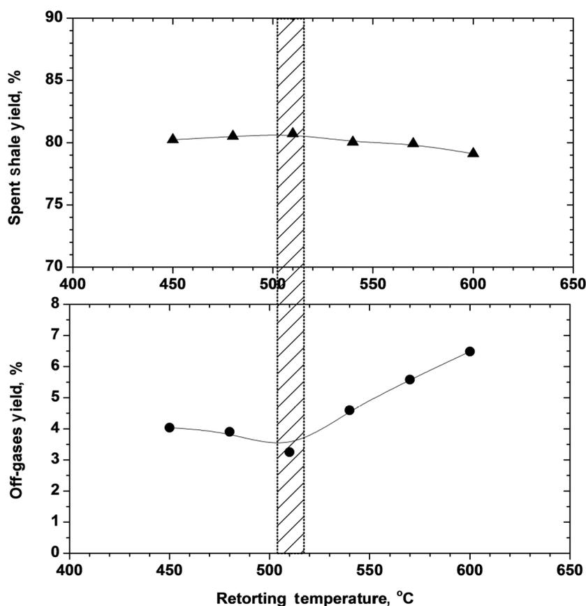
Fig. 3. Change of yield of off-gases and spent shale with retorting temperature (shale particle size 1.4 mm, shale hold time 40 min).
