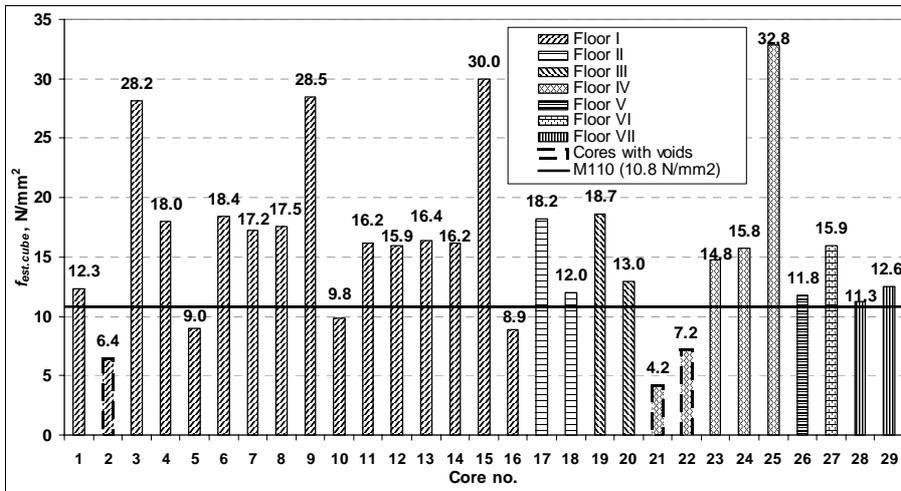
Fig. 4. Compressive strength of 29 cores drilled from columns.
