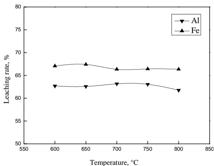
Fig. 5. Influence of calcination temperature of Fushun-type retorting residue on leaching rate of Al and Fe.
