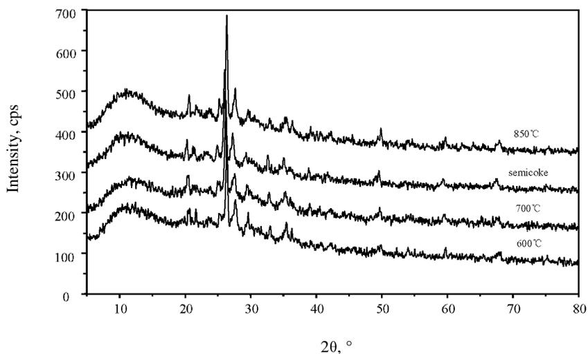
Fig. 2. XRD chart of Fushun-type retorting residue calcined at various temperatures.
