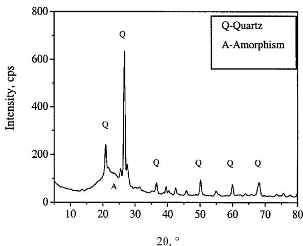
**Fig. 8. XRD chart of separation and purification products.**
