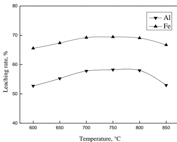
Fig. 4. Influence of calcination temperature of circular retort semicoke on leaching rate of Al and Fe.
