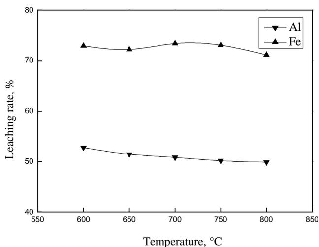
Fig. 6. Influence of calcination temperature of residue from cogeneration plant on leaching rate of Al and Fe.
