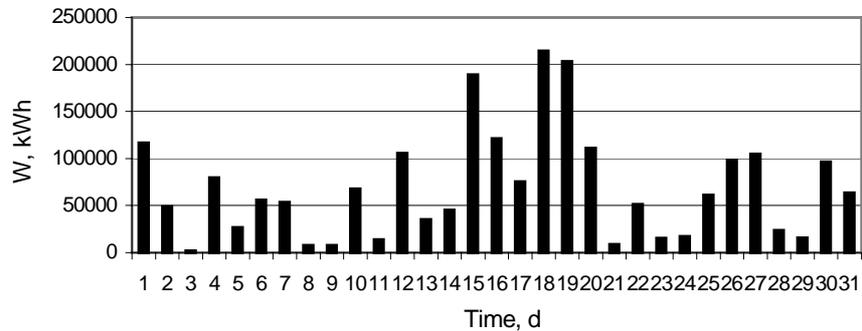
Fig. 5. The daily electric energy production of Pakri wind farm (July, 2006).
