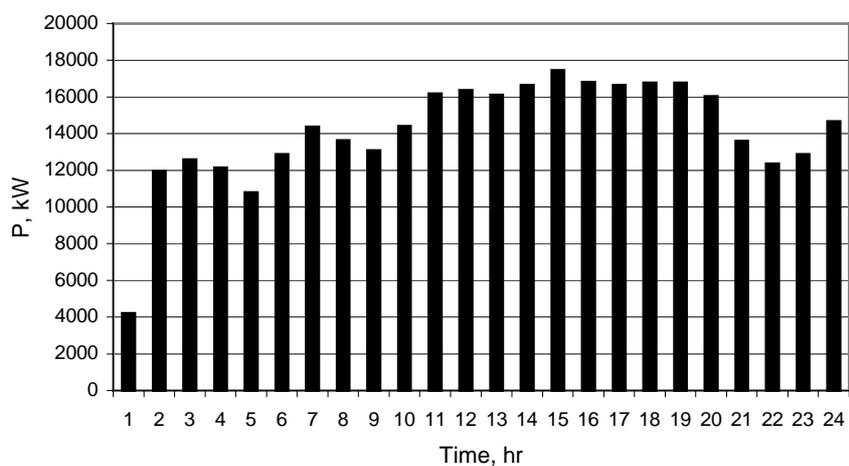
Fig. 9. The hourly theoretical, based on the wind speed, electric energy production of Pakri wind farm (July 18, 2006).
