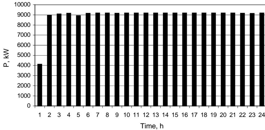
Fig. 8. The hourly electric energy production of Pakri wind farm (July 18, 2006).
