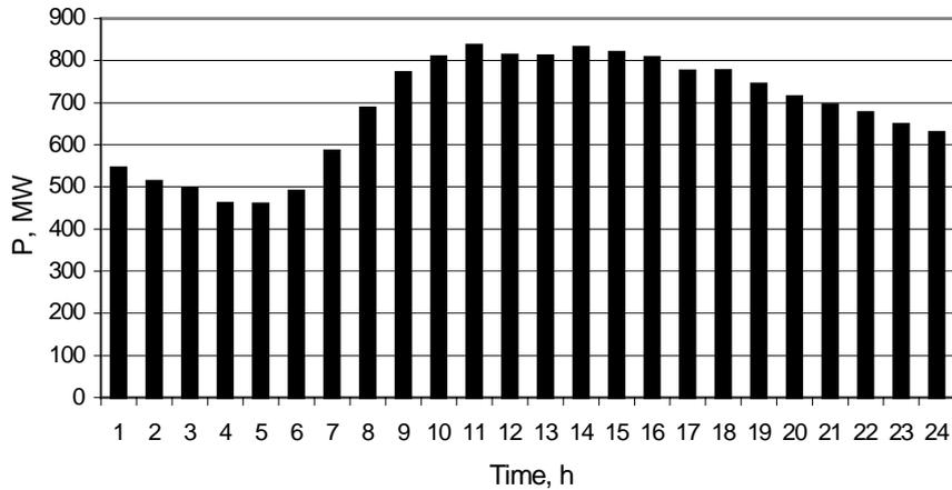
Fig. 7. The load curve of the Estonian energy system (July 3, 2006).
