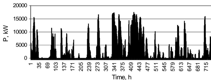
Fig. 4. The possible power load curve of Pakri wind farm (July, 2006).
