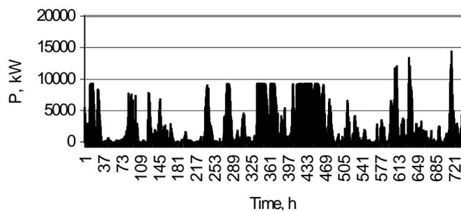
Fig. 3. Power load curve of Pakri wind farm (July, 2006).
