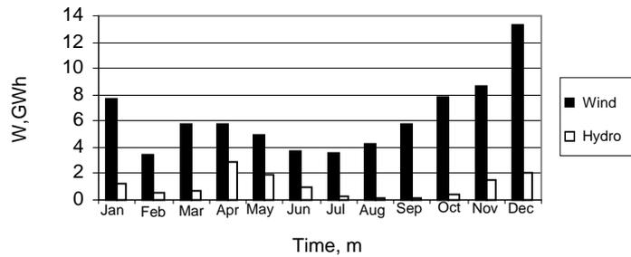
Fig. 2. Load curves of wind and hydroelectric power stations in Estonia (2006).
