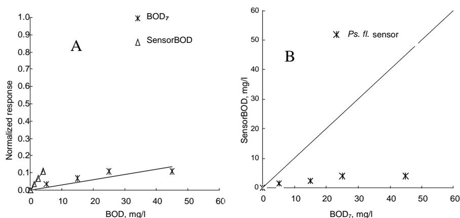
Fig. 6. (A) Comparison of linear range of *Ps. fl.* biosensor measurements with phenol solution, where BOD<sub>7</sub> values for each dilution were calculated from the results obtained from conventional method and sensor-BOD values were obtained from the calibration curve. (B) Correlation of *Ps. fl.* biosensors sensor-BOD to BOD<sub>7</sub> in phenol solution, where the dotted line represents the 1-1 correlation line.
