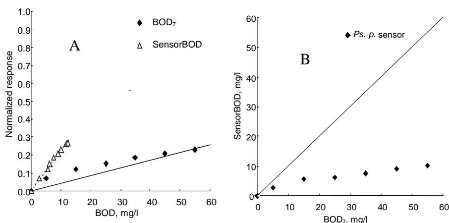
Fig. 5. (A) Comparison of linear range of *Ps. p.* biosensor measurements with phenol solution, where BOD<sub>7</sub> values for each dilution were calculated from the results obtained from standard BOD<sub>7</sub> method and sensor-BOD values were obtained from the calibration curve. (B) Correlation of *Ps. p.* biosensors sensor-BOD to BOD<sub>7</sub> in phenol solution, where the dotted line represents the 1-1 correlation line.
