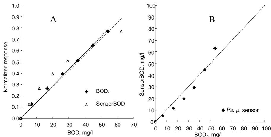
Fig. 3. (A) Comparison of linear range of *Ps. p.* biosensor measurements with phenol-spiked OECD synthetic wastewater, where BOD<sub>7</sub> values for each dilution were calculated from the results obtained from standard BOD<sub>7</sub> method and sensor-BOD values were obtained from the calibration curve. (B) Correlation of *Ps. p.* biosensors sensor-BOD to BOD<sub>7</sub> in phenol-spiked OECD synthetic wastewater, where dotted line represents the 1-1 correlation line.
