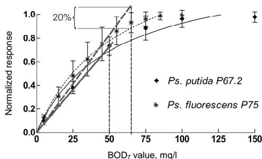
Fig. 2. Calibration curves for *Ps. p.* BOD biosensor and *Ps. fl.* BOD biosensor in OECD synthetic wastewater. Straight lines show the linear approximation of the Michaelis-Menten curves in the region where deviation is less than 20%.
