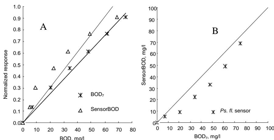
Fig. 4. (A) Comparison of linear range of *Ps. fl.* biosensor measurements with phenol-spiked OECD synthetic wastewater, where BOD<sub>7</sub> values for each dilution were calculated from the results obtained from standard BOD<sub>7</sub> method and sensor-BOD values were obtained from the calibration curve. (B) Correlation of *Ps. fl.* biosensors sensor-BOD to BOD<sub>7</sub> in phenol-spiked OECD synthetic wastewater, where the dotted line represents the 1-1 correlation line.
