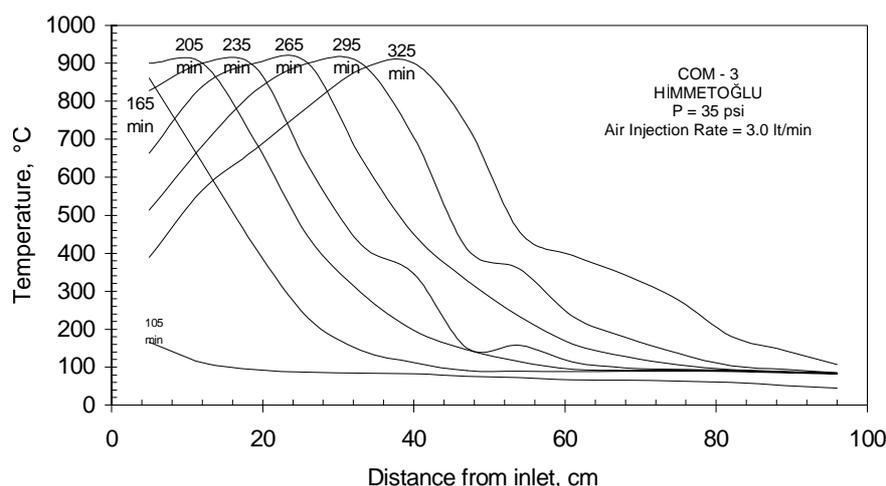
Fig. 2. Temperature profile along combustion tube (Himmetoğlu oil shale).
