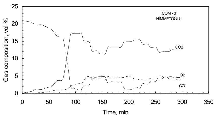
Fig. 4. Composition of produced gas vs. time (Himmetoğlu oil shale).
