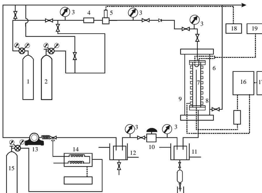
Fig. 1. Schematic diagram of the combustion tube apparatus.
