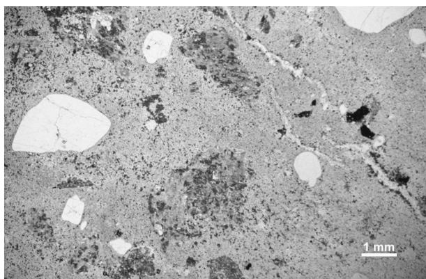
**Fig. 3.** Suursaari quartz porphyry: quartz and turbid orthoclase phenocrysts in submicroscopic groundmass. Thin-section, back-scattered image. Sample S-32, Mäkiinpäällys.
