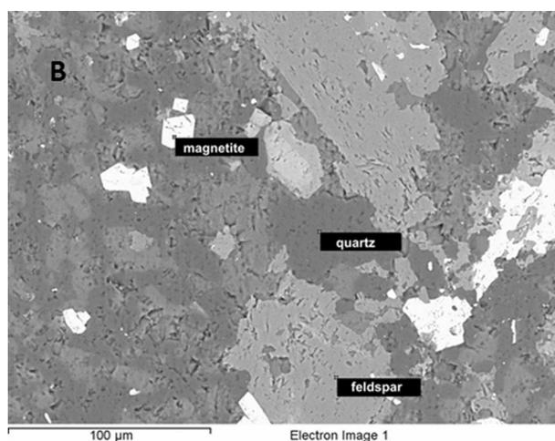
**Fig. 4.** Suursaari quartz porphyry: magnetite, orthoclase and plagioclase inclusions in quartz phenocryst. Sample S-32, Mäkiinpäällys. Quartz phenocrysts in Suursaari quartz porphyrite contain some accessory minerals: magnetite (A, B), feldspar (B) and plagioclase (A). Scanning electron microscope (SEM) images.
