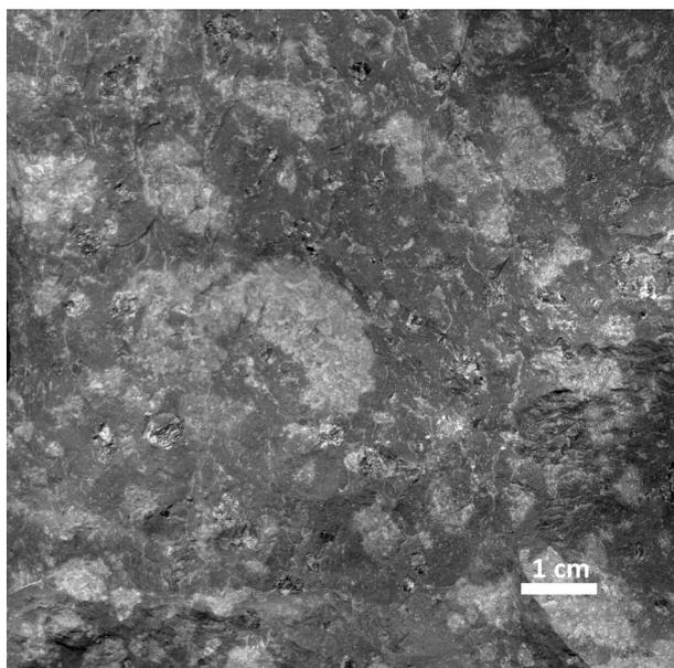
**Fig. 2.** Suursaari quartz porphyry: quartz and orthoclase phenocrysts (light) in aphanitic groundmass (dark). Sample S-32, Mäkiinpäällys.
