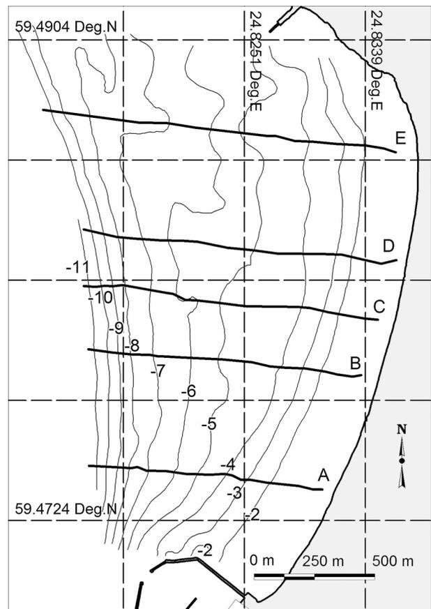
**Fig. 11.** Bathymetry of the nearshore of Pirita Beach according to the water depth survey in April 2006. The water depth along profiles A–E is given in Fig. 12. The coastline is shown based on the digital 1 : 50 000 Estonian Base Map from the Estonian Land Board ([www.maaamet.ee](http://www.maaamet.ee)).
