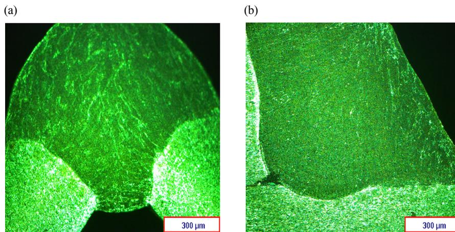
Fig. 3. Micrographs of the cross-sections of welds: (a) corner joint  $Q(H) = 0.081$  kJ/mm; (b) T-joint  $Q(H) = 0.107$  kJ/mm.
