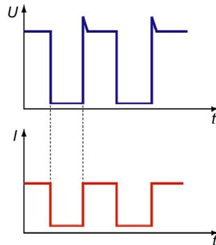
**Fig. 1.** Arc voltage and current in the CMT process.
