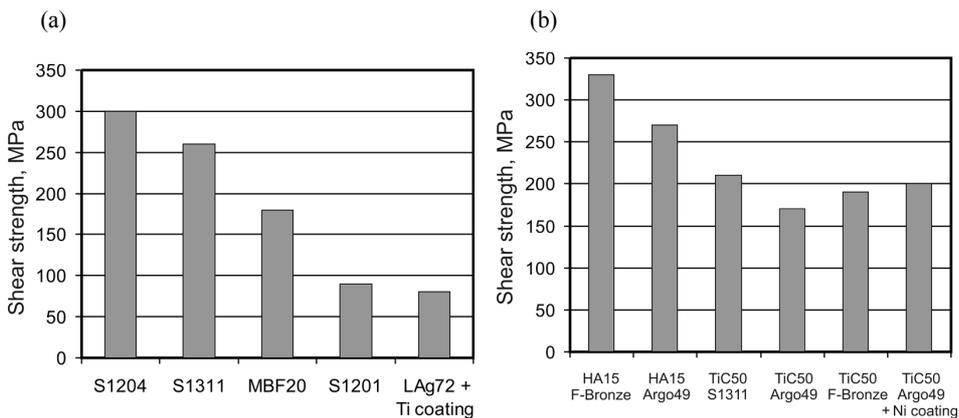
**Fig. 4.** Shear strength of TiC-based cermets and reference WC-based hardmetal, brazed to structural steel: (a) vacuum brazing, cermet TiC60/FeNi; (b) air brazing, cermet TiC50/NiMo and hardmetal HA15.
