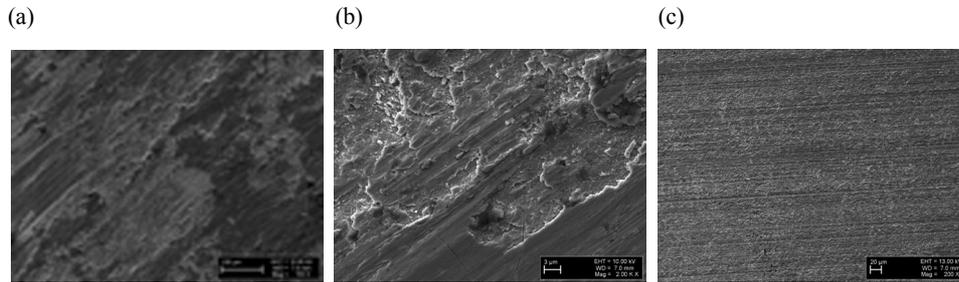
**Fig. 2.** SEM photographs of the metallized surface: (a), (b) mechanically metallized Ti-coating; (c) electrochemical Ni coating.
