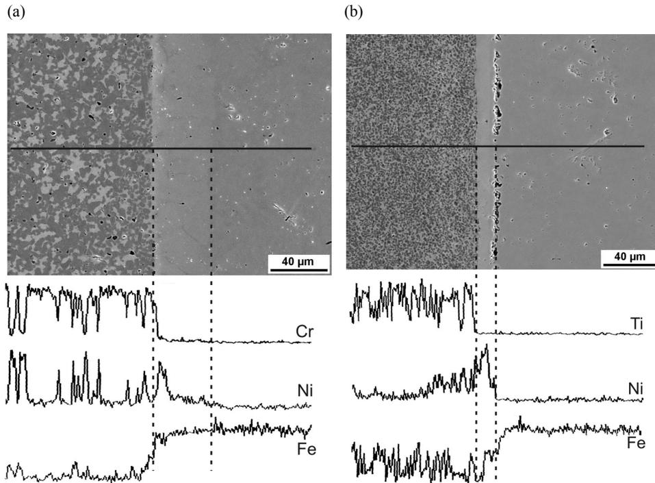
**Fig. 5.** Structure and element distribution of vacuum brazed joints using amorphous filler metal S1311: (a) CrNi30 cermet; (b) TiC50/NiMo cermet.
