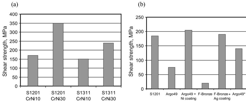
**Fig. 3.** Shear strength of joints “chromium carbide-based cermets + steel”: (a) brazing in vacuum, counterpart–structural steel; (b) brazing in air, counterpart–structural steel, \* counterpart–stainless steel.
