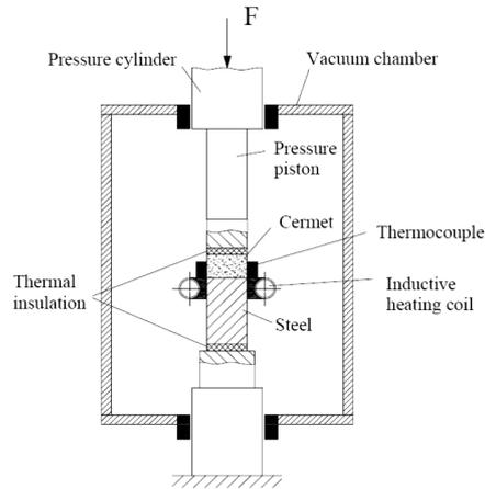
**Fig. 1.** Schematic diagram of a vacuum bonding hot press.
