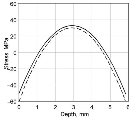
**Fig. 3.** Principal stress profiles through the panel thickness at a point on the symmetry axis of a tempered glass panel of thickness 6 mm: (—)  $\sigma_1$ , (---)  $\sigma_2$ .
