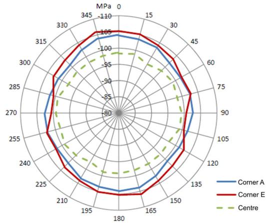
**Fig. 10.** Directional variation of the surface residual stress at the centre and at the points A and E.
