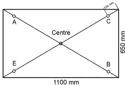
**Fig. 9.** Geometry of a tempered glass panel. According to European standards the stresses are to be measured at the centre and at the four corners.
