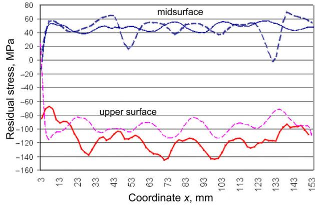
**Fig. 5.** Distribution near the edge of  $\sigma_x$  on the  $x$  axis in panel No. 1 (— calculated, - - - measured).
