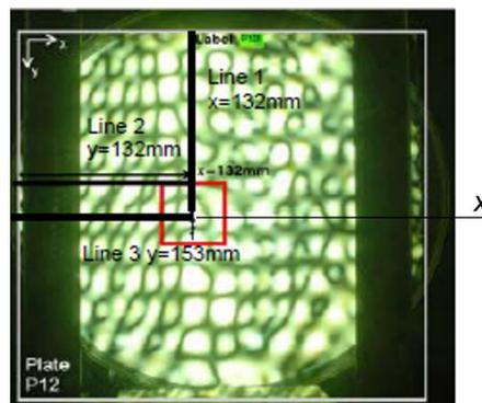
**Fig. 4.** Photoelastic fringe pattern of the panel No. 1.
