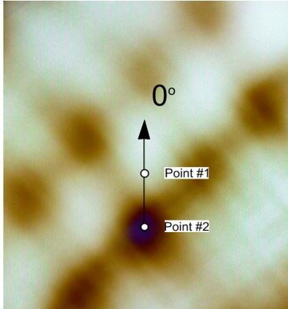
**Fig. 7.** Interference pattern in a circular polariscope of the central part of a sidelite.
