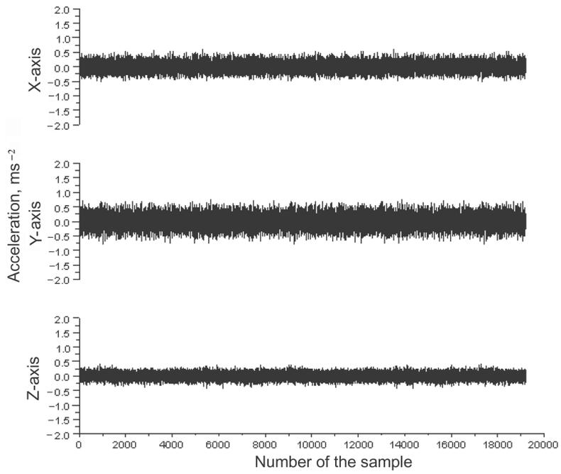
**Fig. 1.** Noise floor level test No. 1.
