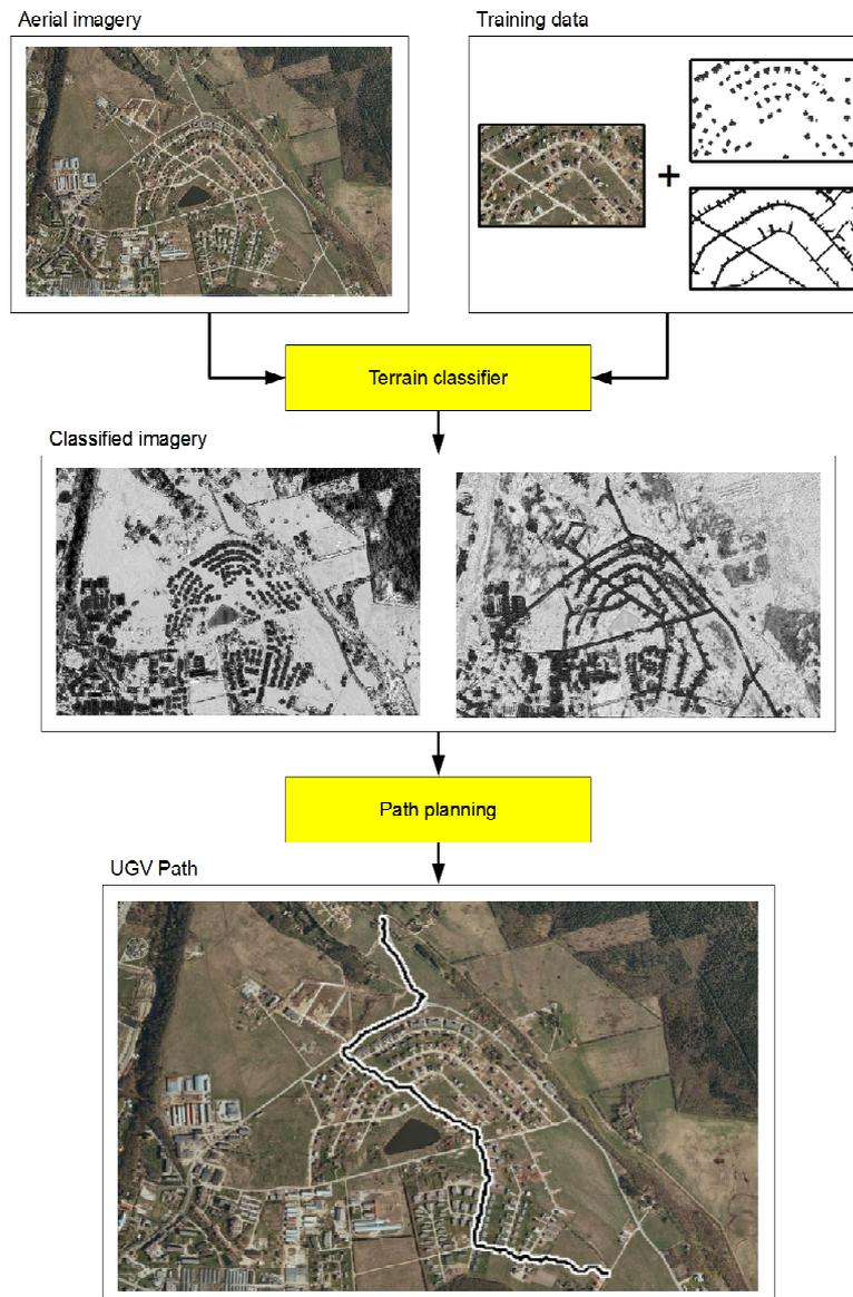
**Fig. 1.** Terrain classification and path planning.
