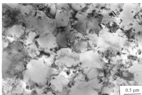
Fig. 1. Substructure of initial Al- \text{Al}_4\text{C}_3 material with 4 vol% of \text{Al}_4\text{C}_3 (transverse direction).
