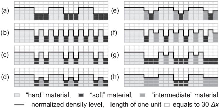
**Fig. 2.** Substructure compositions. The bold line describes the relative density of the material. The light grey layers represent the material of the bar ( $\rho = 4510 \text{ kg/m}^3$ ,  $c = 5240 \text{ m/s}$ ), shaded layers indicate the “intermediate” substructure material ( $\rho = 3603 \text{ kg/m}^3$ ,  $c = 5100 \text{ m/s}$ ) and the dark grey layers – the “soft” substructure material ( $\rho = 2703 \text{ kg/m}^3$  and  $c = 5020 \text{ m/s}$ ).
