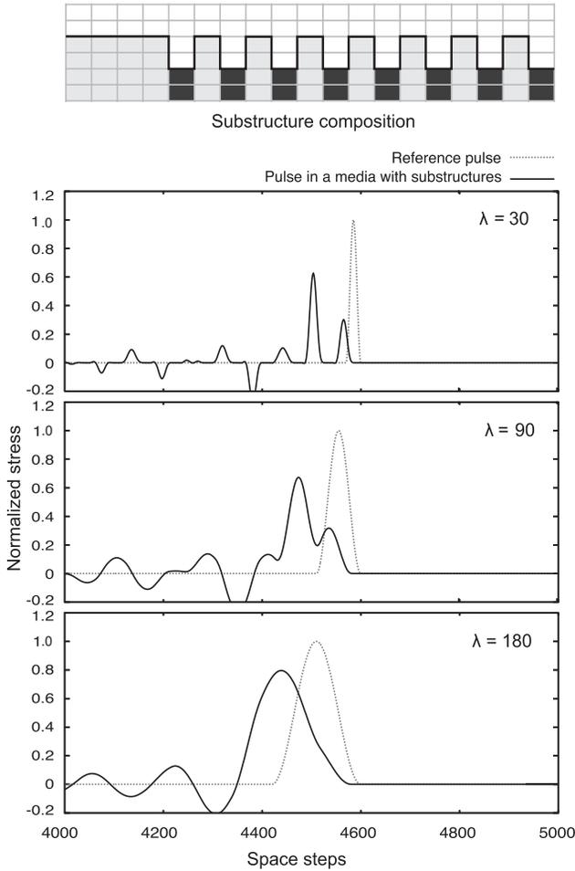
**Fig. 4.** Pulse shape at 4600 time steps for “hard–soft” structure laminate ( $d = 30\Delta x$ , case (b) in Fig. 2).
