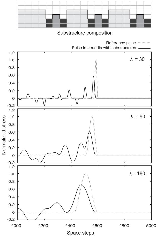
**Fig. 6.** Pulse shape at 4600 time steps for “hard–soft–intermediate–soft” double structure laminate ( $d = 30\Delta x$  and  $90\Delta x$ , case (d) in Fig. 2).
