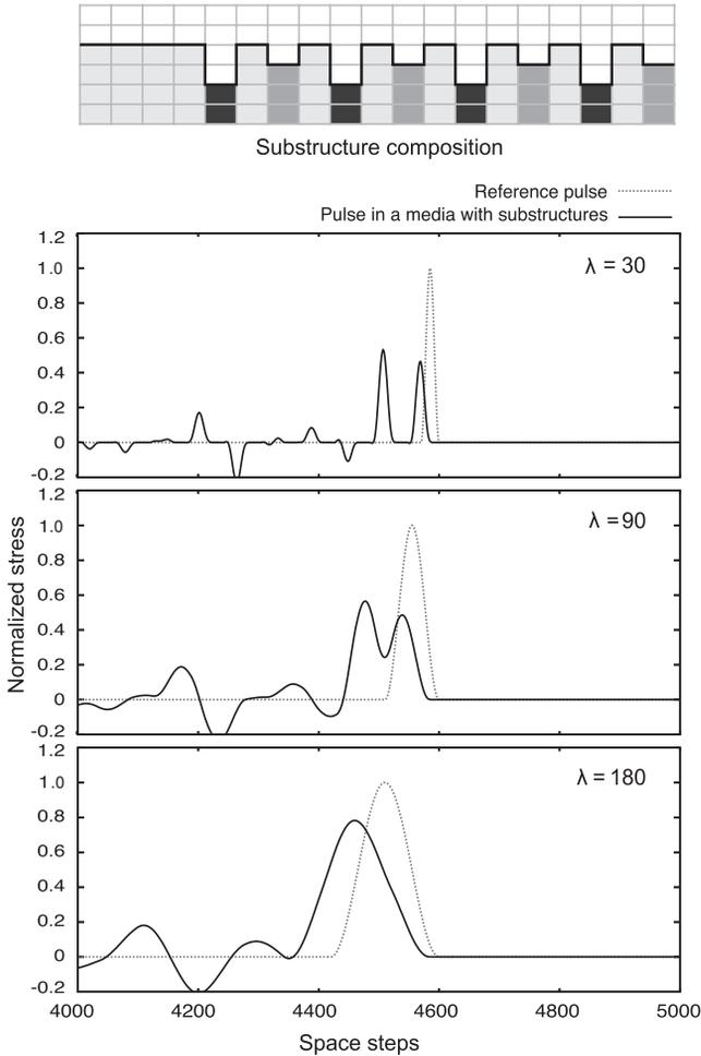
**Fig. 8.** Pulse shape at 4600 time steps for “hard–soft–hard–intermediate” double structure laminate ( $d = 30\Delta x$ , case (f) in Fig. 2).
