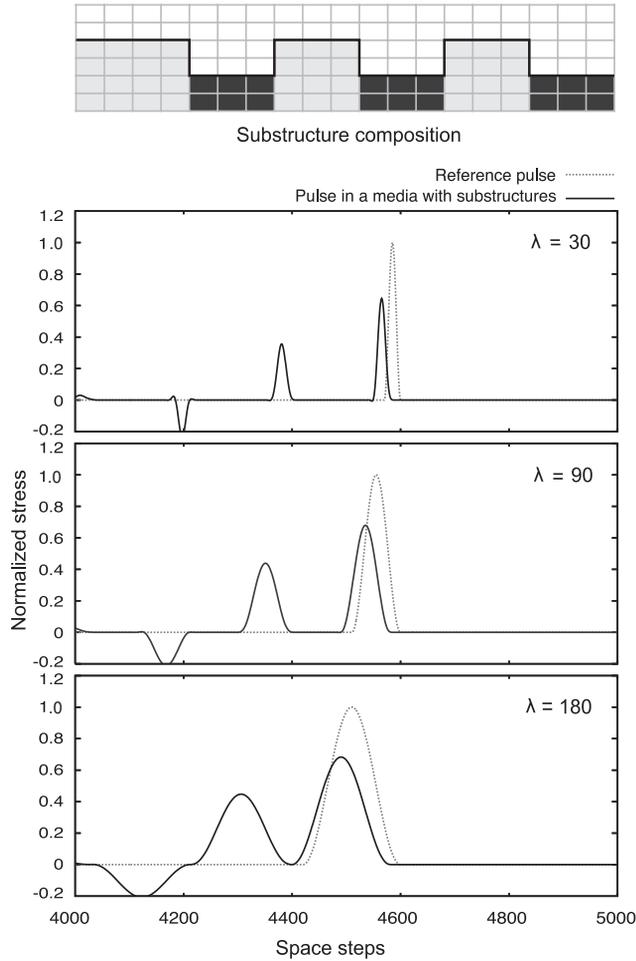
**Fig. 3.** Pulse shape at 4600 time steps for “hard–soft” structure laminate ( $d = 90\Delta x$ , case (a) in Fig. 2).
