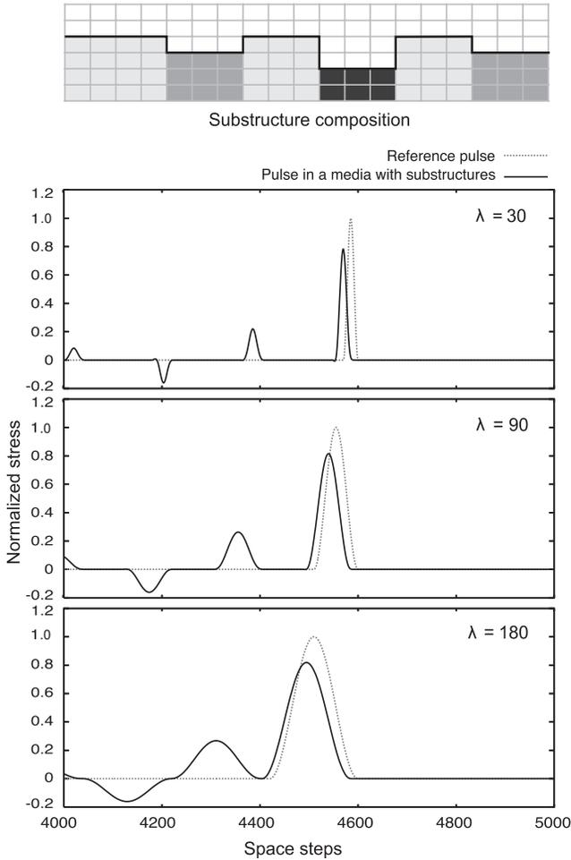
**Fig. 10.** Pulse shape at 4600 time steps for “hard–intermediate–hard–soft” double structure laminate ( $d = 90\Delta x$ , case (h) in Fig. 2).
