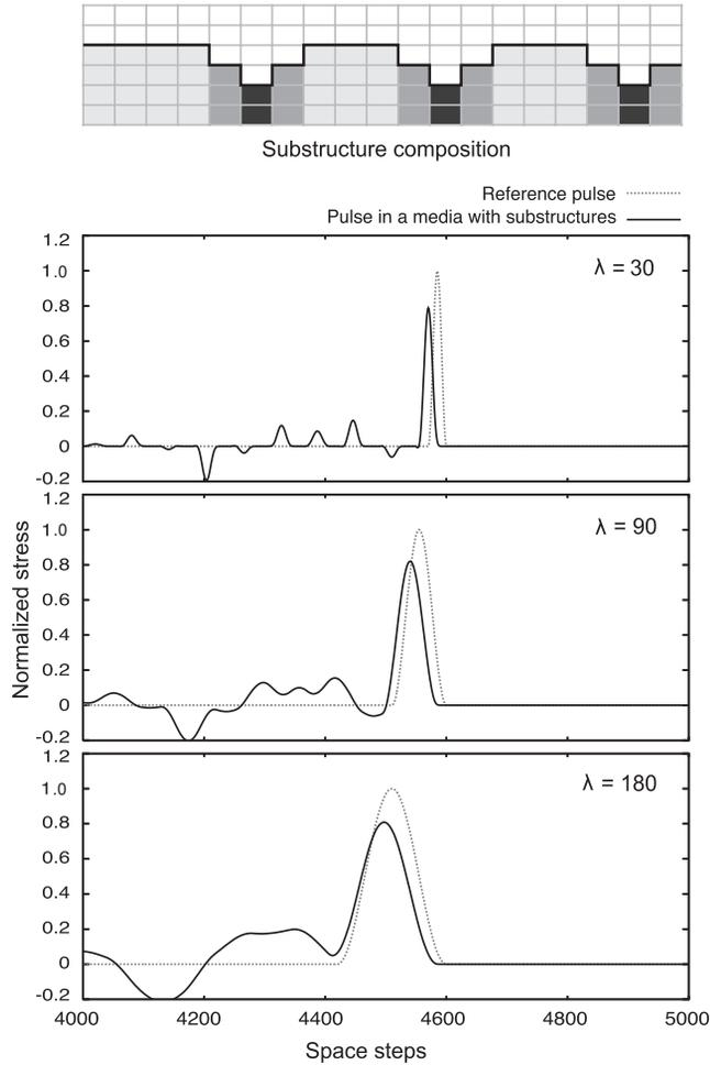
**Fig. 7.** Pulse shape at 4600 time steps for “hard–intermediate–soft–intermediate” double structure laminate ( $d = 30\Delta x$  and  $90\Delta x$ , case (e) in Fig. 2).
