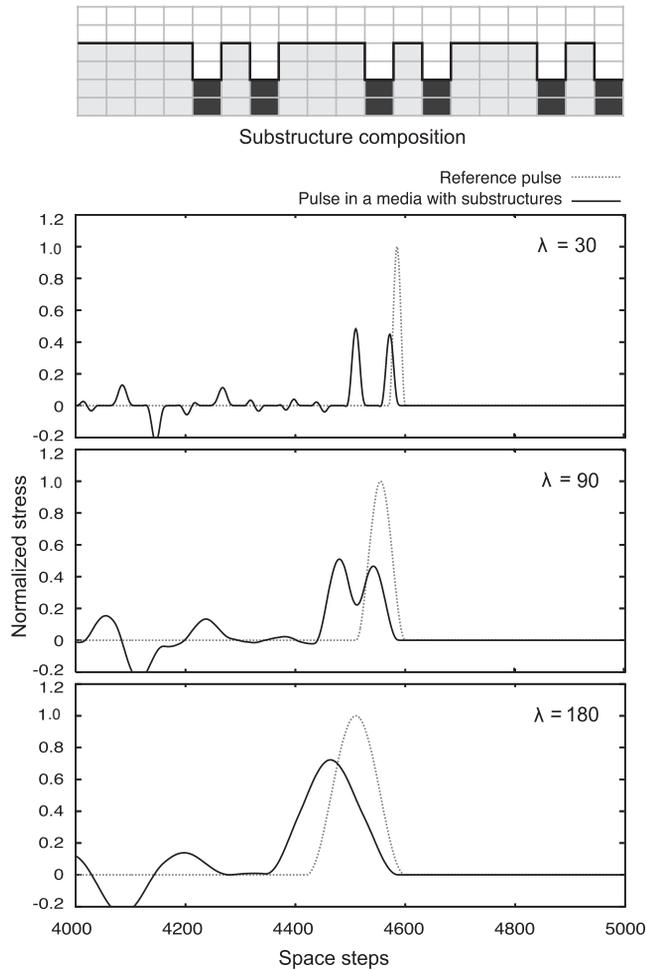
**Fig. 5.** Pulse shape at 4600 time steps for mixed “hard–soft” structure laminate ( $d = 30\Delta x$  and  $90\Delta x$ , case (c) in Fig. 2).
