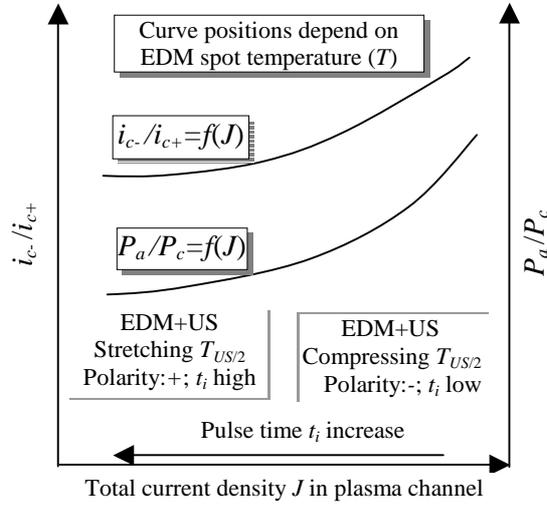
**Fig. 1.** Qualitative variation of working parameters influencing electrode wear.
