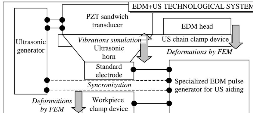
**Fig. 4.** CIM system for EDM+US.
