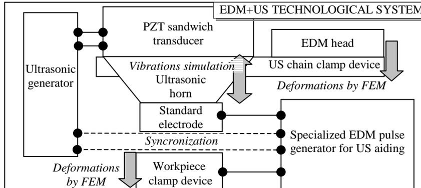
Fig. 4. CIM system for EDM+US.
