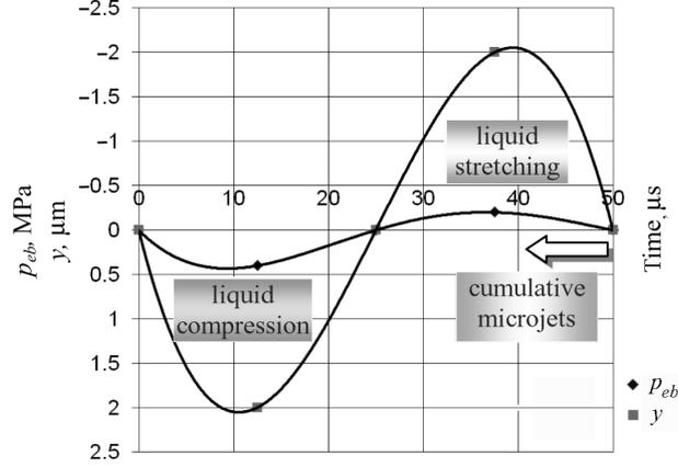
Fig. 3. Cavitation phenomena ultrasonically induced at EDM+US.
