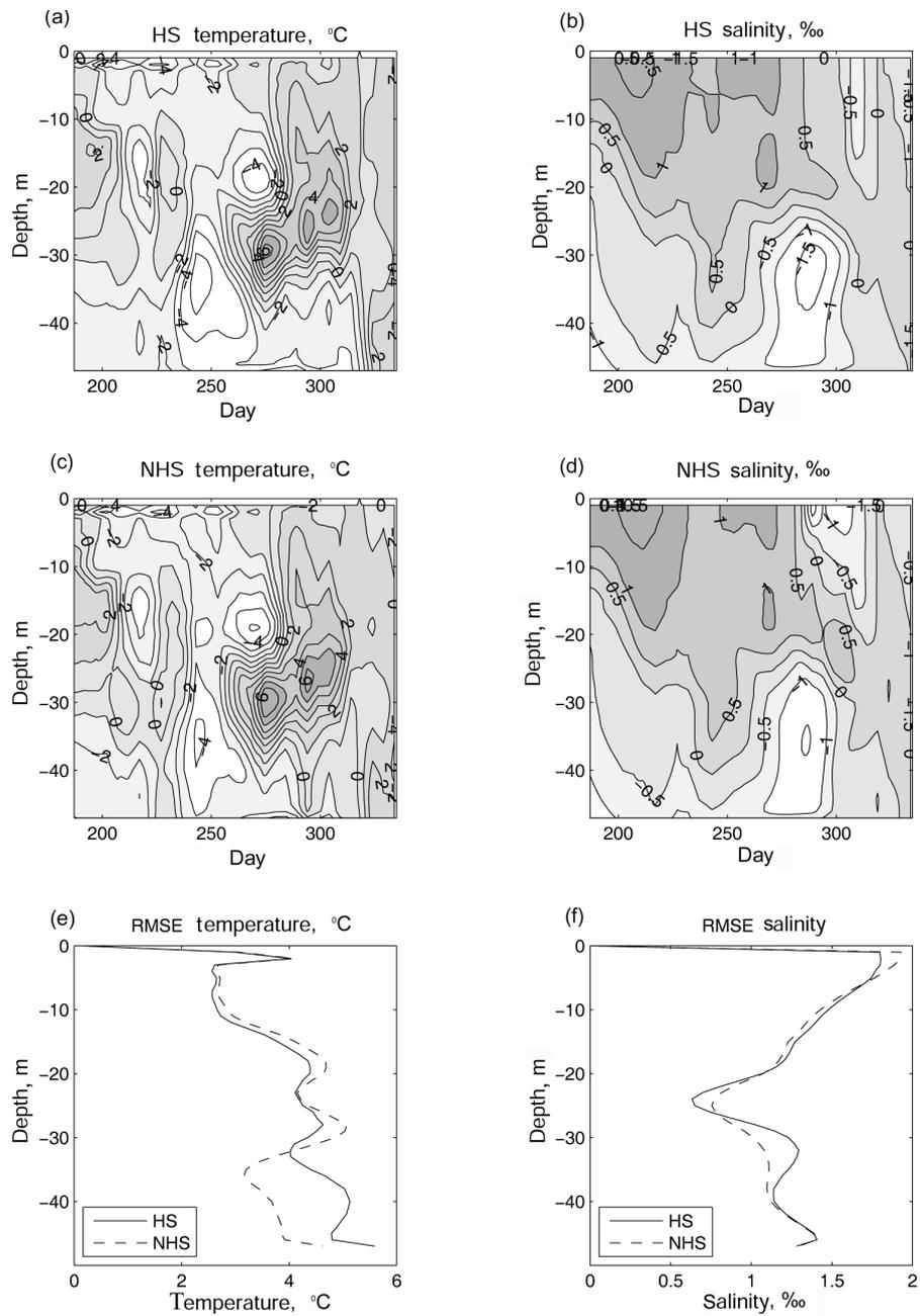
**Fig. 5.** Difference between the measurement data and model results at the Huovari monitoring station: HS temperature (a) and salinity (b), NHS temperature (c) and salinity (d), RMSE for temperature (e) and salinity (f). The measurement data were made available by the Eutrophication-Maps project [21].
