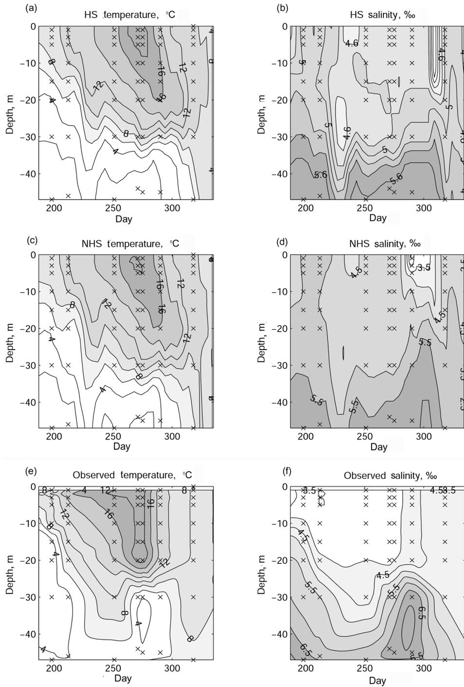
**Fig. 3.** Modelled HS temperature (a) and salinity (b), NHS temperature (c) and salinity (d) and observed temperature (e) and salinity (f) at the Huovari monitoring station. The measurement data were made available by the Eutrophication-Maps project [21].
