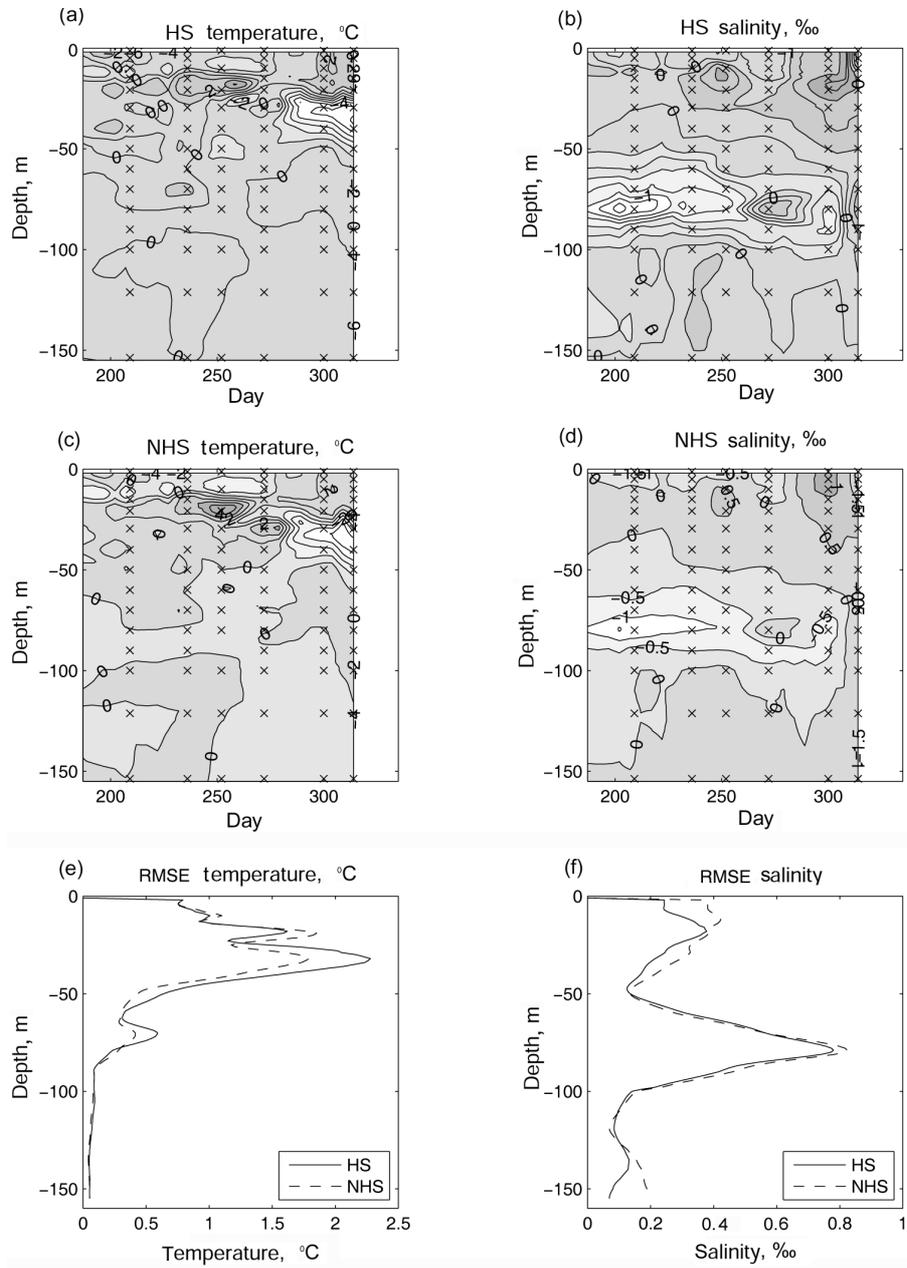
**Fig. 6.** Difference between the measurement data and model results at the monitoring station BY29: HS temperature (a) and salinity (b), NHS temperature (c) and salinity (d), RMSE for temperature (e) and salinity (f). The measurement data were made available by the Eutrophication-Maps project [21].
