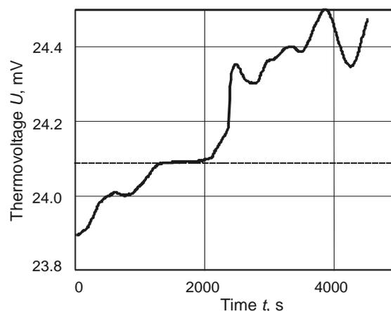
**Fig. 12.** Single typical thermovoltage behaviour from Fig. 11 during a calibration process with superposed process-dependent temperature variations (thermocouple type K).
