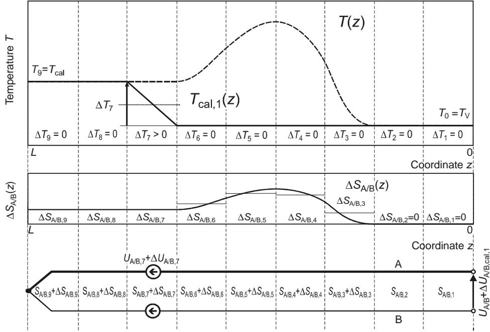
**Fig. 5.** Equivalent circuit of the inhomogeneous thermocouple according to Fig. 4 with temperature-dependent inhomogeneities (inhomogeneously distributed drift portions  $\Delta S_{A/B,i}$  and  $\Delta U_{A/B,i}$ ) in sections 3 to 9 at a calibration temperature profile  $T_{cal,1}(z)$  with an effective temperature gradient in section 7.
