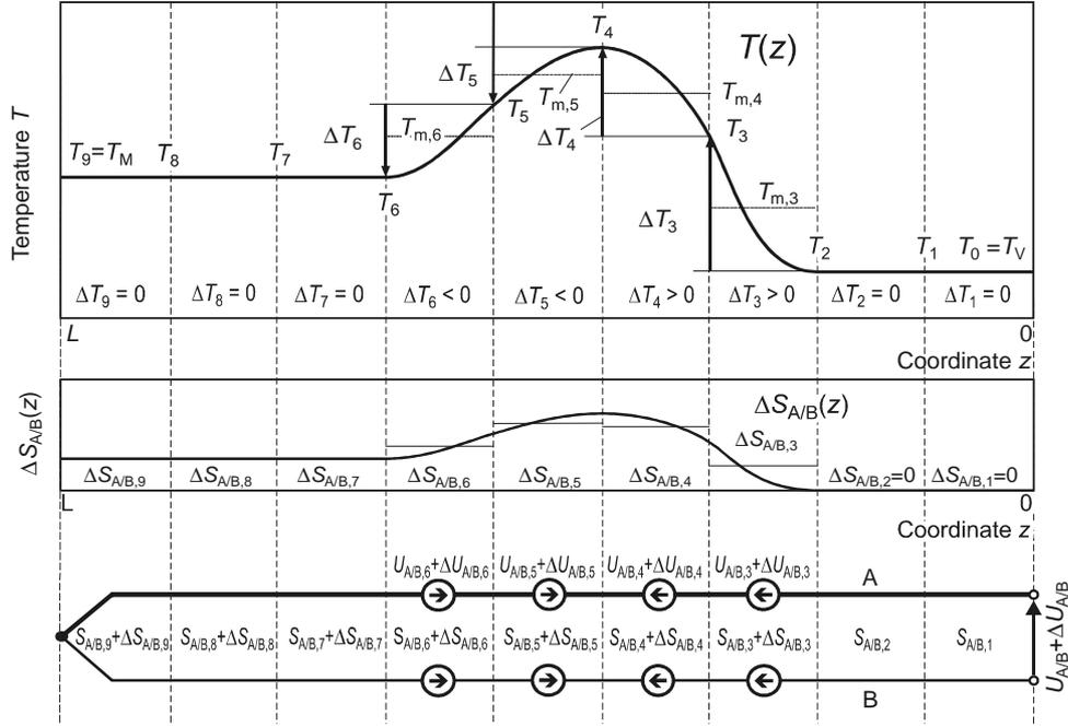
**Fig. 4.** Equivalent circuit of the thermocouple according to Fig. 1 with temperature-dependent inhomogeneities (inhomogeneously distributed drift portions  $\Delta S_{A/B,i}$  and  $\Delta U_{A/B,i}$ ) in sections 3 to 9 and effective temperature gradient in sections 3 to 6.
