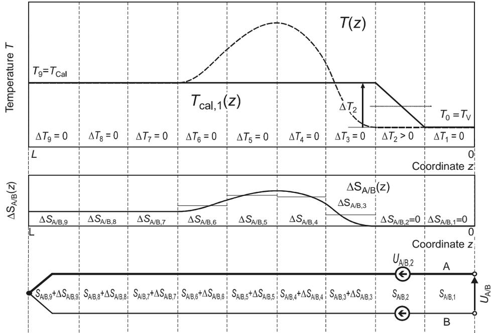
**Fig. 6.** Equivalent circuit of the inhomogeneous thermocouple according to Fig. 4 with temperature-dependent inhomogeneities (inhomogeneously distributed drift portions  $\Delta S_{A/B,i}$  and  $\Delta U_{A/B,i}$ ) in sections 3 to 9 at a calibration temperature profile  $T_{cal,2}(z)$  with an effective temperature gradient in section 2.
