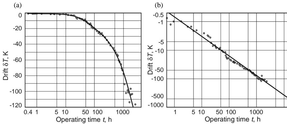
**Fig. 3.** Ageing of a NiCr-NiAl thermocouple (type K, 0.8 mm  $\varnothing$ ) at an operating temperature of  $T_M = 850^\circ\text{C}$  [9]: (a) linear scale; (b) logarithmic scale.
