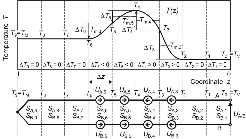
**Fig. 1.** Schematic, illustrating the gradient theory of the emergence of the thermovoltage: equivalent circuit of a thermocouple, made of the materials A and B at a temperature profile  $T(z)$  with effective temperature gradients in the sections 3 to 6.
