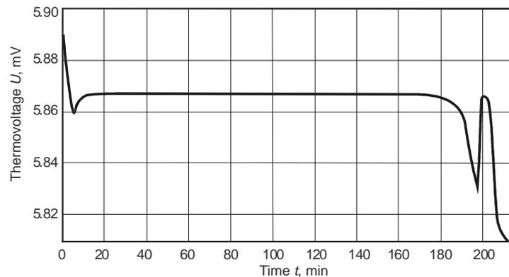
**Fig. 15.** Freezing plateaus of a reference aluminium fixed-point cell ( $T_{FP} = 660.323^\circ\text{C}$ ) and of the aluminium miniature fixed-point cell in the MFP-thermocouple type N after long-time operation at steam temperatures of  $630^\circ\text{C}$ .
