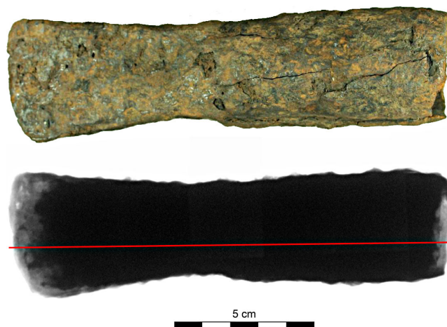
Fig. 3. The Kohtla axe (TÜ 2309: 203) before cutting. The cutting path is marked on the X-ray. X-ray settings: 50 kV, 4 mA, 8 s, brass filter (X-ray by Kristiina Paavel).
