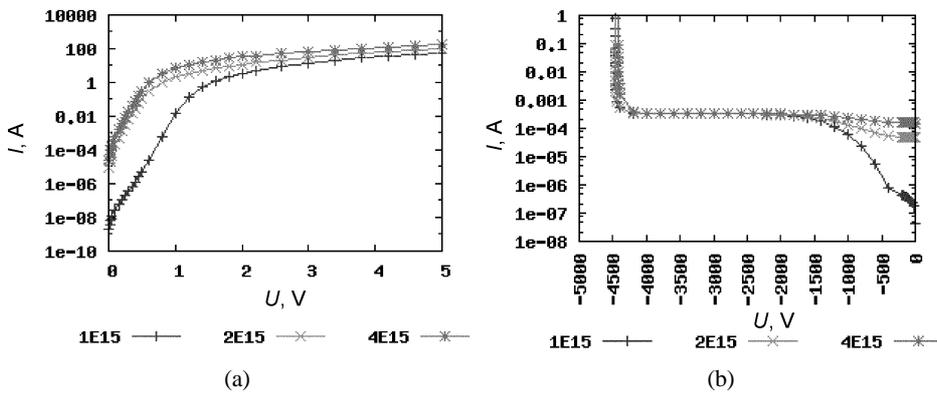
**Fig. 13.** Dependence of the forward (a) and reverse (b) characteristics on the doping concentration of the epitaxial layer.
