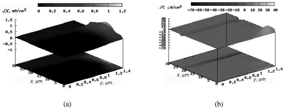
**Fig. 5.** Values of the  $x$  (a) and  $y$  (b) components of the density of the reverse current in the device "1.5-10-0.5" at 1000 V reverse voltage; current density direction is opposite to the direction of the  $x$  axis.
