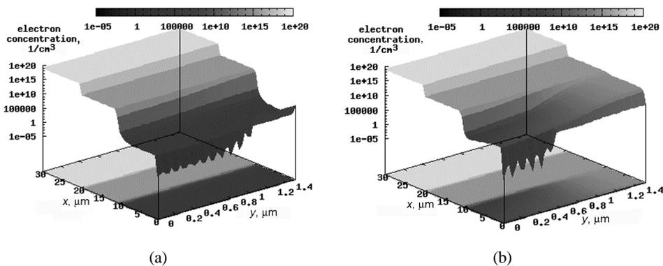
**Fig. 2.** Electron concentration in devices “1.5-10-1” (a) and “1.5-10-0.5” (b) for at 0.3 V forward voltage.
