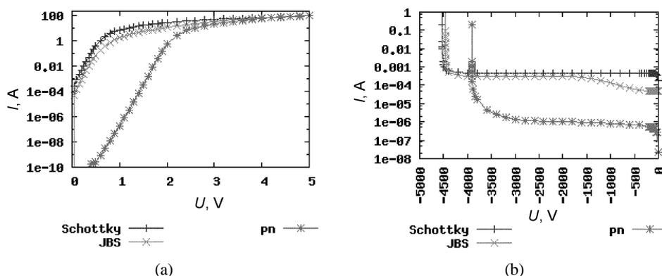
Fig. 17. Forward (a) and reverse (b) characteristics of the Schottky, JBS and  $pn$ -diodes.
