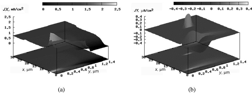
**Fig. 6.** Values of the  $x$  (a) and  $y$  (b) components of the density of the reverse current in the device “1.5-10-1” at 1000 V reverse voltage; current density direction is opposite to the direction of the  $x$  axis.
