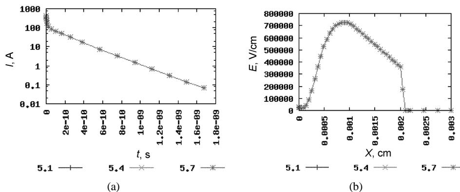
Fig. 16. Dependence of the turn-off characteristics (a) and electric field strength distribution (b) on the contact metal work function.
