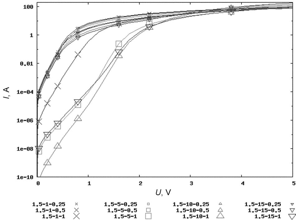
**Fig. 1.** Forward  $U$ - $I$  characteristics of JBS devices with different deepness and width of the emitter area; legend shows width of the whole structure, deepness of the emitter and width of the emitter in  $\mu\text{m}$ .
