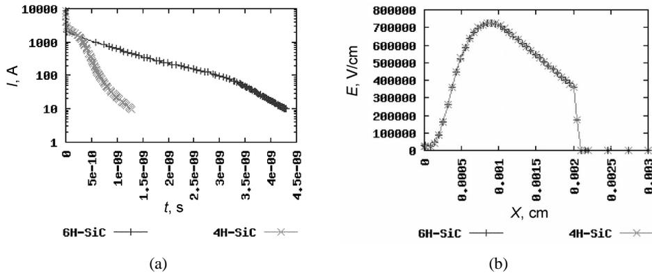
**Fig. 12.** The turn-off characteristics (a) and distribution of the electric field strength (b) in 6H-SiC and 4H-SiC JBS devices.
