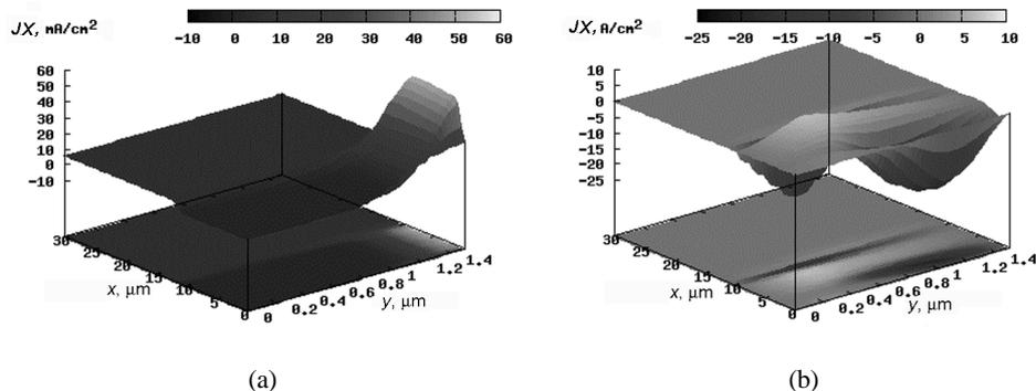
**Fig. 3.** Values of the  $x$  (a) and  $y$  (b) components in the device “1.5-10-0.5” at 0.3 V forward voltage; direction of the current density is opposite to the direction of the  $x$  axis.
