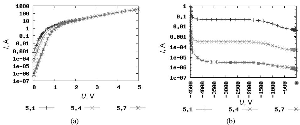
Fig. 15. Dependence of the forward (a) and reverse (b) characteristics on the contact metal work function.
