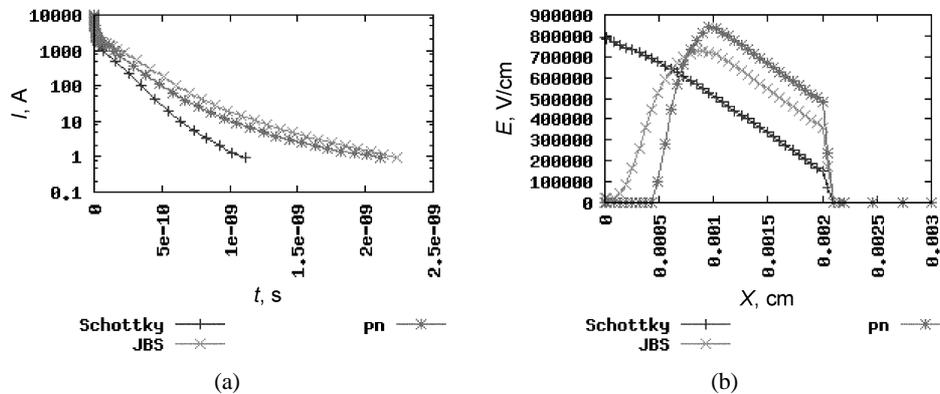
**Fig. 18.** Distribution of the turn-off characteristics (a) and electric field strength (b) in Schottky, JBS and  $pn$ -diodes.
