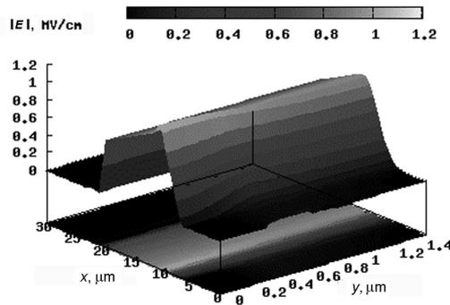
**Fig. 8.** Electric field distribution at reverse voltage 1000 V in case of the device “1.5-10-0.5”.
