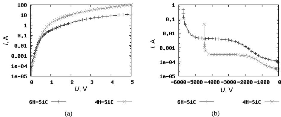
Fig. 11. Forward (a) and reverse (b)  $U$ - $I$  characteristics of 6H-SiC and 4H-SiC.
