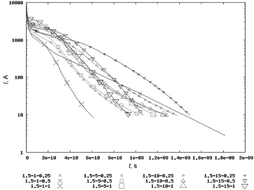
**Fig. 9.** Turn-off current switching JBS from 100 A to  $-100$  V with different emitter deepness and width; legend shows width of the whole structure and deepness and width of the emitter in  $\mu\text{m}$ .
