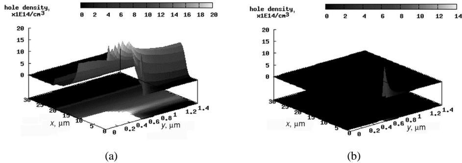
**Fig. 10.** Hole density at forward voltage 5 V: (a) device “1.5-10-0.5” (emitter area hole concentration is out of the range and not shown); (b) device “1.5-1-0.5”.
