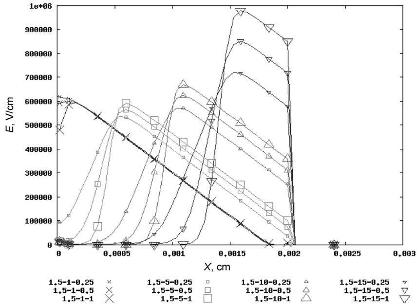
**Fig. 7.** Distribution of the electric field under Schottky contact of JBS devices with different emitter deepness and width; legend shows width of the whole structure and deepness and width of the emitter in  $\mu\text{m}$ .
