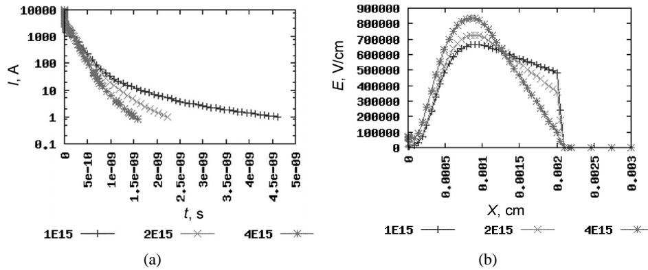
**Fig. 14.** Dependence of the turn-off characteristics (a) and electric field distribution (b) on the doping concentration of the epitaxial layer.
