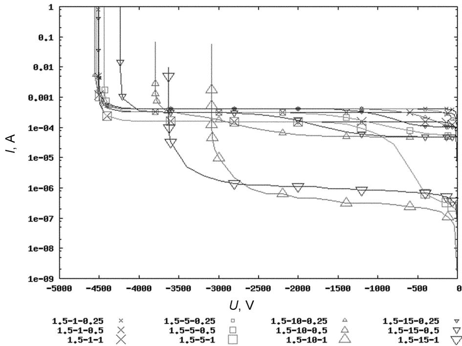
**Fig. 4.** Reverse  $U$ - $I$  characteristics of JBS devices with different deepness and width of the  $p$  doping area; legend shows width of the whole structure and deepness and width of the  $p$  doping area in  $\mu\text{m}$ .
