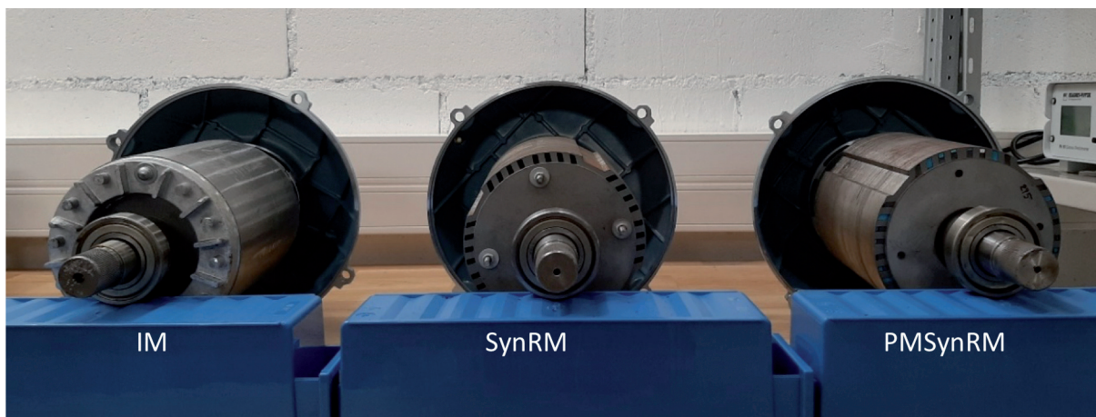
Fig. 2. Rotors of the tested electrical machines front view.
