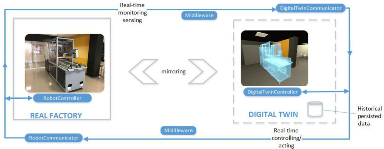
Fig. 2. Synchronization process through the proposed software infrastructure.
