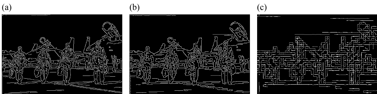
Fig. 10. The example of an image with MD where the Canny edge detection operator was applied to three levels of decomposition for the Haar wavelet transformation. (a) Level 1, (b) Level 2, (c) Level 3.
