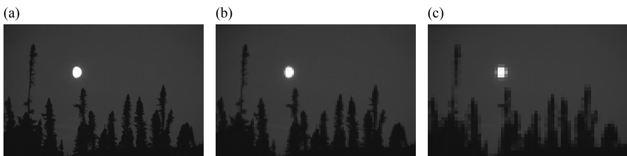
Fig. 6. The example of an image with LD where the Haar wavelet transformation is applied to three levels of decomposition. (a) Level 1, (b) Level 2, (c) Level 3.
