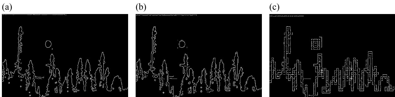
Fig. 9. The example of an image with LD where the Canny edge detection operator was applied to three levels of decomposition for the Haar wavelet transformation. (a) Level 1, (b) Level 2, (c) Level 3.
