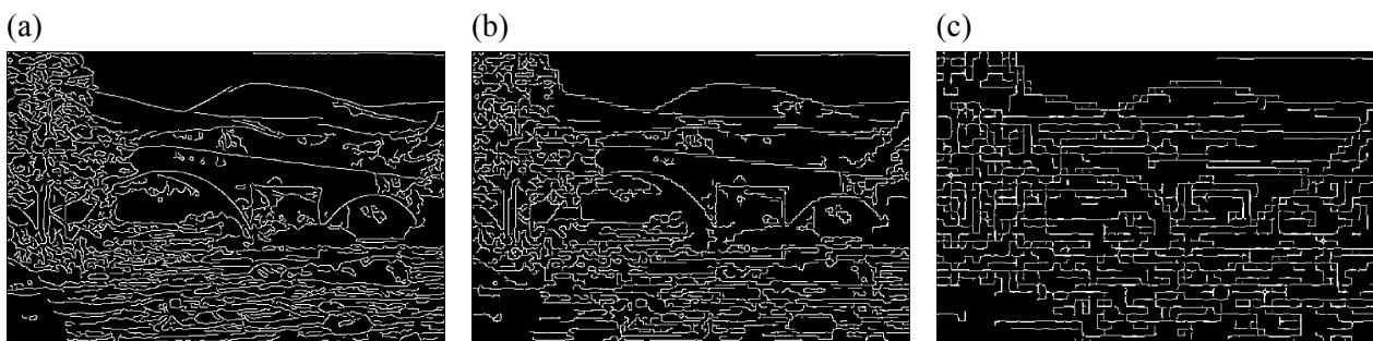
Fig. 11. The example of an image with HD where the Canny edge detection operator was applied to three levels of decomposition for the Haar wavelet transformation. (a) Level 1, (b) Level 2, (c) Level 3.
