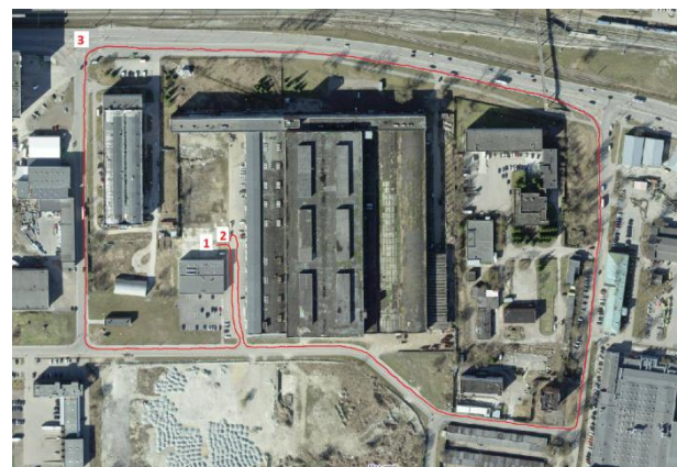
Fig. 12. Route around a defined guarded area of a territory surveillance test with Tracdron recorded by GPS (1 – start, 2 – stop, 3 – pause).
