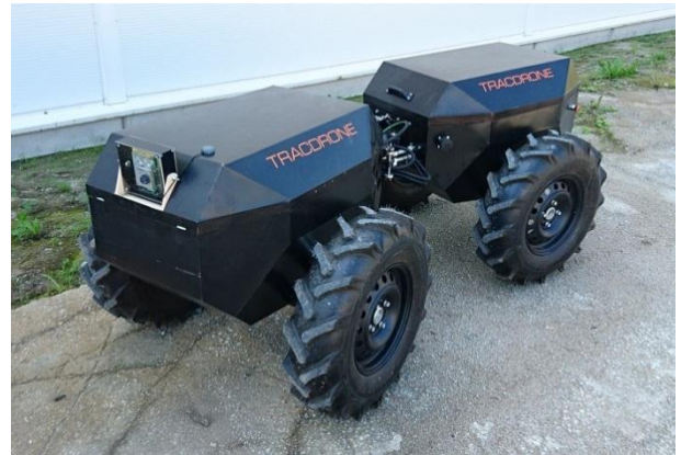
Fig. 2. Electric UGV Tracdron with articulated steering and hydraulic drive.
