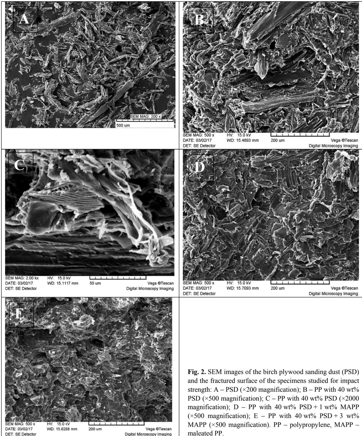
**Fig. 2.** SEM images of the birch plywood sanding dust (PSD) and the fractured surface of the specimens studied for impact strength: A – PSD ( $\times 200$  magnification); B – PP with 40 wt% PSD ( $\times 500$  magnification); C – PP with 40 wt% PSD ( $\times 2000$  magnification); D – PP with 40 wt% PSD + 1 wt% MAPP ( $\times 500$  magnification); E – PP with 40 wt% PSD + 3 wt% MAPP ( $\times 500$  magnification). PP – polypropylene, MAPP – maleated PP.
