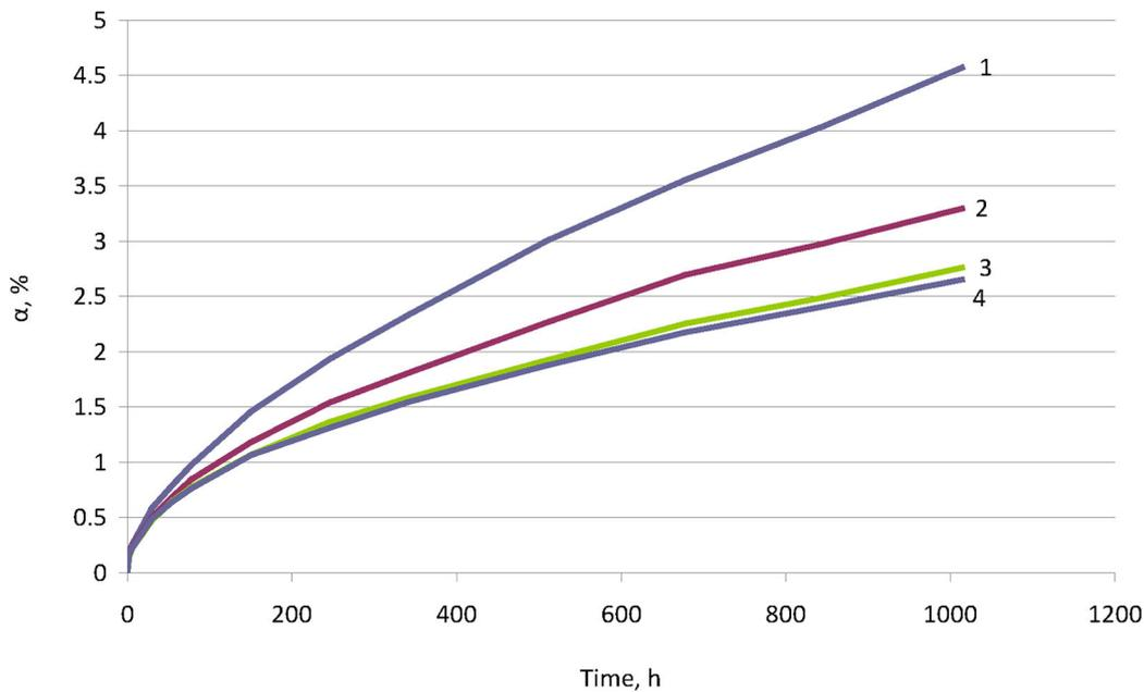
**Fig. 1.** Water absorption kinetics of the polypropylene (PP) composites: 1 – PP + 40 wt% PSD, 2 – PP + 40 wt% PSD + 1 wt% MAPP, 3 – PP + 40 wt% PSD + 3 wt% MAPP, 4 – PP + 40 wt% PSD + 5 wt% MAPP. PSD – birch plywood sanding dust, MAPP – maleated PP.
