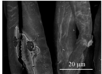
**Fig. 4.** TEOS 4 wt% and ZAD 2.5 wt% coated cotton, mixing/dipping at room temperature.
