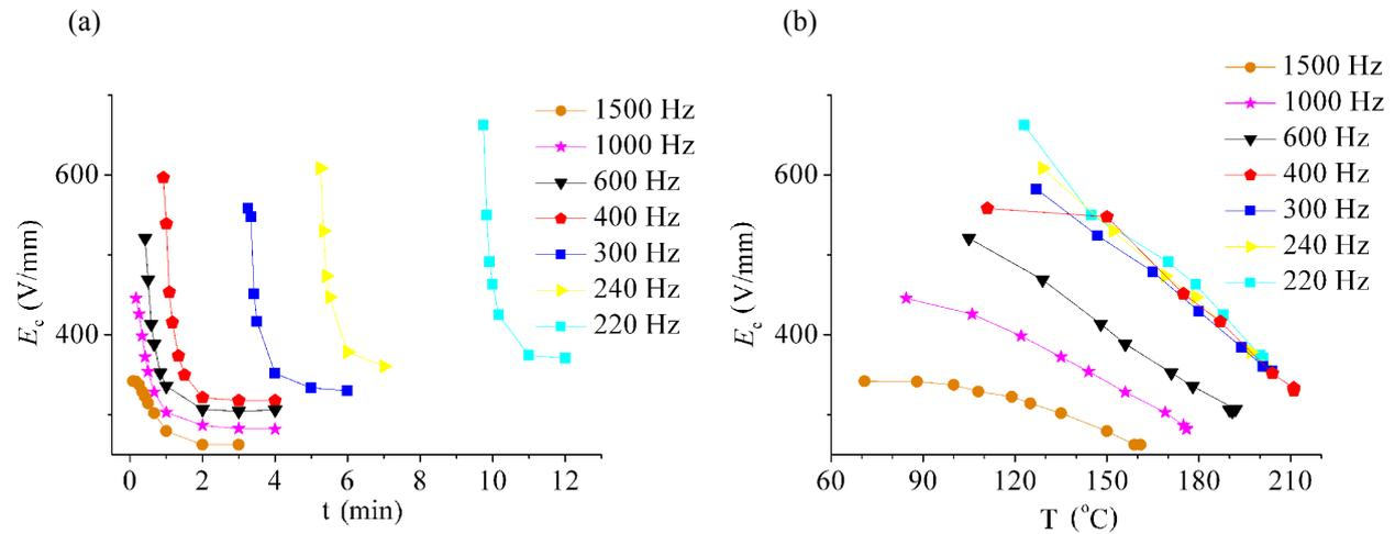
**Fig. 3.** Coercive field time (a) and temperature dependence of PZT sample; (b) during self-heating in electric field of different frequencies.  $E_a = 850$  V/mm.
