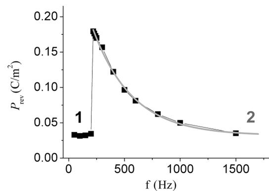
**Fig. 4.** Dependence of the switchable polarization value on frequency (curve 1 – experiment, curve 2 – calculation).  $E_a = 840$  V/mm.
