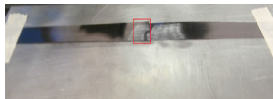
Fig. 2. Test piece. The red rectangle indicates the location of the contact area between two tapes.
