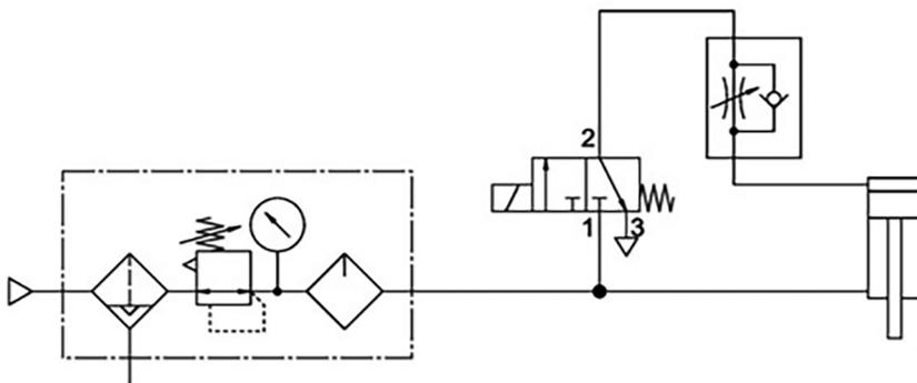
Fig. 5. Schematic representation of the pneumatic system.
