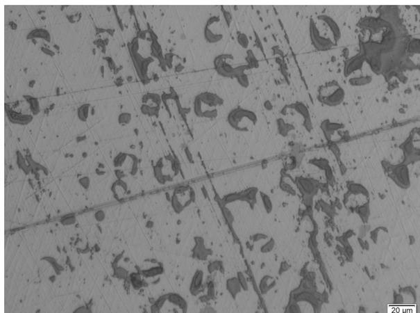
**Fig. 8.** Dots of ink on polished aluminium. The print presents sharp features. Long lines are due to scratches on the aluminium.
