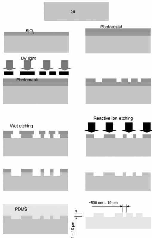
**Fig. 2.** Creation of Si and polydimethylsiloxane (PDMS) stamps. The silicon stamp is created with traditional photolithography methods. PDMS rubber is then poured on the master stamp, providing an exact negative of the silicon stamp.
