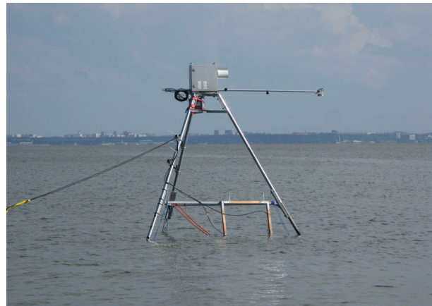
(b) A LOG_aLevel echosounder mounted on top of a tripod
