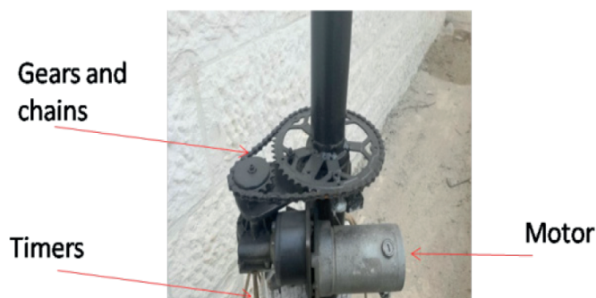
Fig. 3. Solar single-axis tracking system.
