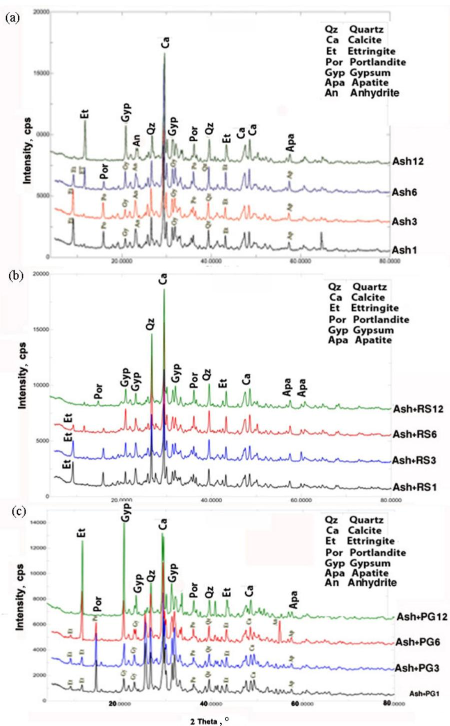
Fig. 4. Overlaid XRD charts for mixtures of all ageing periods: a) ash; b) ash + RS; c) ash + PG.
