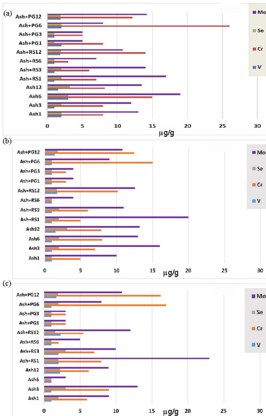
Fig. 3. Histograms showing the effect of pH of solution on the leachability of toxic elements from all studied mixtures of all ageing periods: a) pH 5; b) pH 7; c) pH 9.
