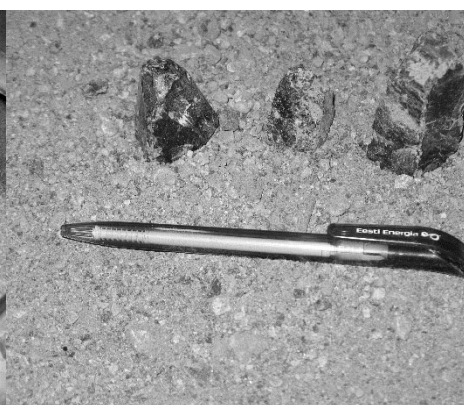
Fig. 6. Oversized coal pieces in the fuel blend.
