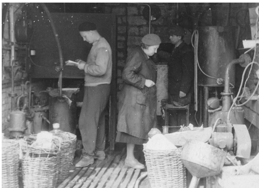
Fig. 2. Periodical-cycle dicarboxylic acids units at Kiviõli Oil Shale Chemical Integrated Plant: a 74-litre oxidation reactor and the nitric acid “storage” (on the left), a vacuum distillation device and a dichloroethane “storage” for extraction of raw dicarboxylic acids (on the right). Junior researcher Rein Veski recording the data, Aleksandra Fomina, head of the laboratory of high-molecular compounds of the Institute of Chemistry, Estonian SSR Academy of Sciences, watching the progress of the oxidation experiment and junior researcher Aleksandr Iljin holding manually the pressure in the reactor at the required level.
