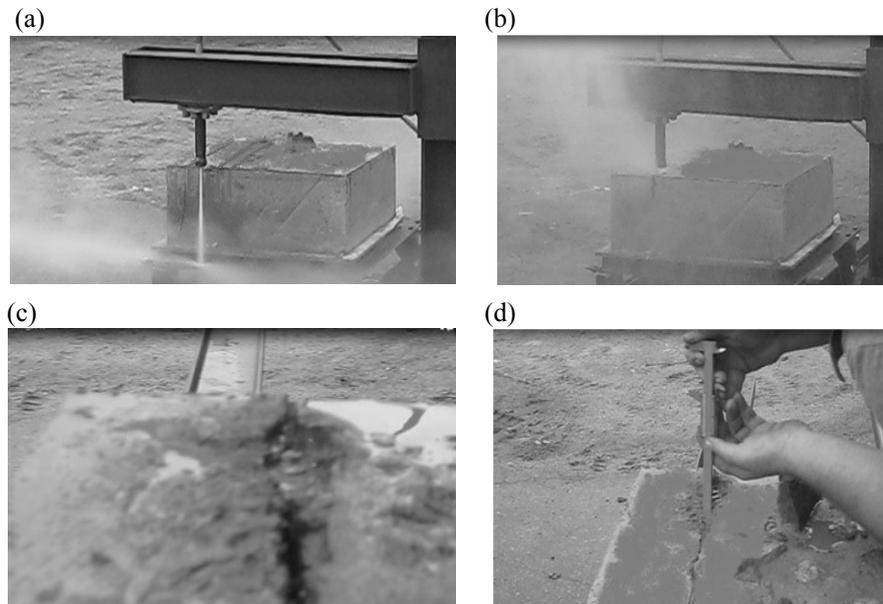
Fig. 2. Oil shale cutting by high-pressure water jets: a) before cutting; b) cutting; c) cut; d) measurement of the depth of cut.
