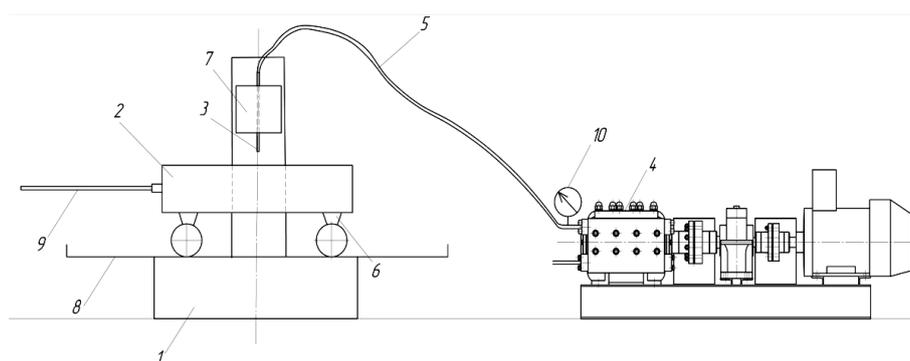
Fig. 1. Scheme of testing equipment: 1 – the frame; 2 – the oil shale sample; 3 – the jet forming device; 4 – the pump; 5 – the high pressure hose; 6 – the movable table; 7 – the holder; 8 – the guiding units; 9 – the cable; 10 – the manometer.
