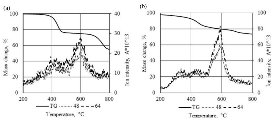
Fig. The release of  $\text{SO}_2$  during thermal decomposition of samples: (a) Estonian oil shale, (b) Chinese oil shale.
