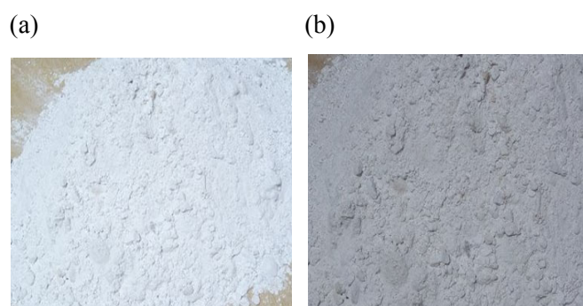
Fig. 1. Dry granite (a) and marble (b) wastes samples.
