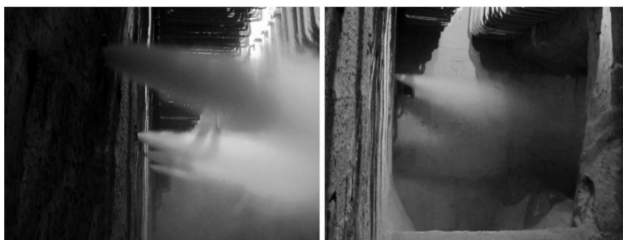
Fig. 4. Photos of the injection of technical water during cold tests in the boiler.
