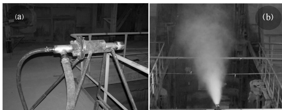
Fig. 3. (a) Connection of the vapour sprayers with pressurised air and water hoses; (b) one of the regimes of the pre-settings of the vapour sprayers (water pressure 4 bar, air pressure 2 bar, the position of the thread regulating the cone of the water spray is minimal).
