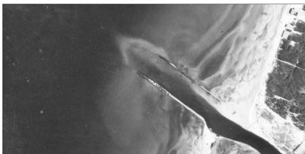
**Fig. 6.** The Pirita River mouth in 1951 (detail of the photo in Fig. 5) illustrating the joint effect of groins along the river coasts and the river flow on the formation of the sand bar at the end of the groins.
