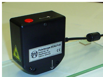
Fig. 3. Surface stress measurement with the scattered light polariscope (left) and thickness stress distribution near the surface (right).
