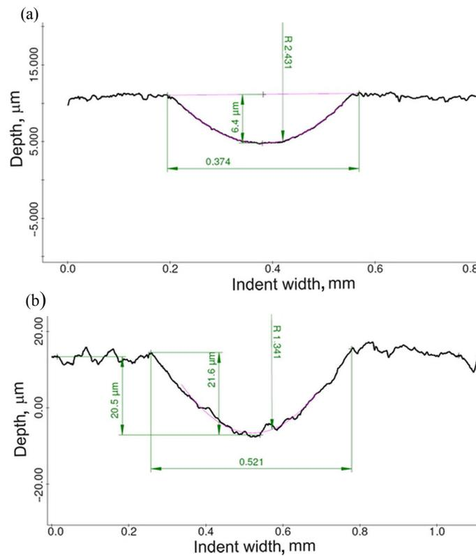
**Fig. 3.** Indents cross-section dimensions of HARDOX 400 (a) and C60E (b) steels for 300 N indentation load.
