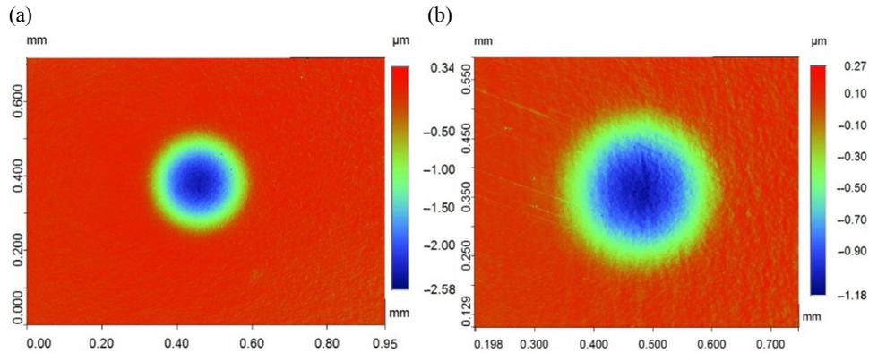
**Fig. 5.** Indents morphologies of H15 hardmetal (a) and T30A cermet (b) for indentation load of 300 N.
