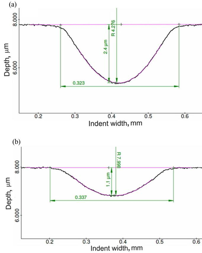
**Fig. 4.** Indents cross-section dimensions of H15 hardmetal (a) and T30A cermet (b) for 300 N indentation load.
