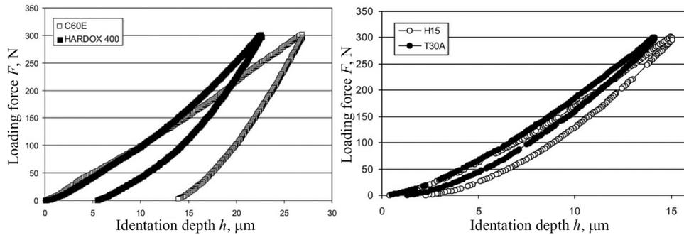
**Fig. 2.** Spherical indentation curves for studied materials.
