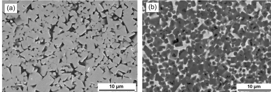
**Fig. 1.** SEM micrographs of the tested H15 (a) and T30A (b) carbide composite.
