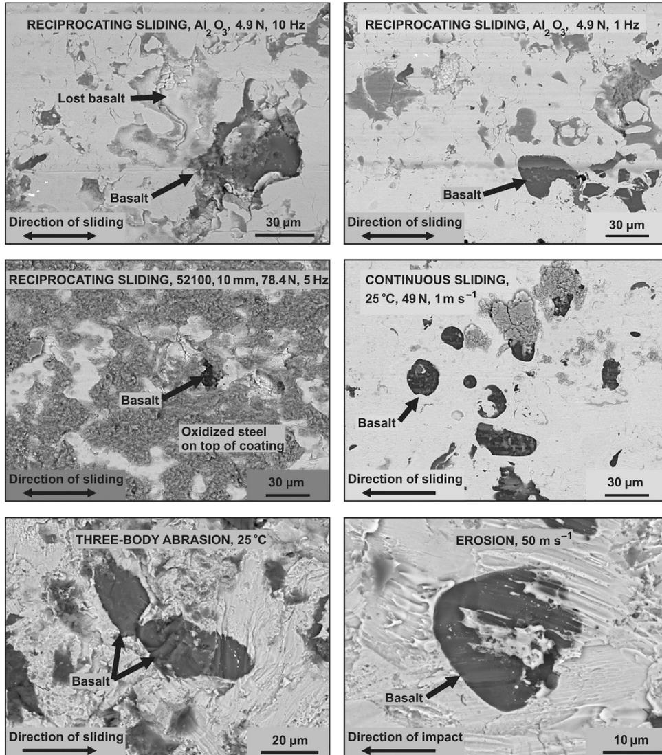
Fig. 5. Backscattered SEM images of the FeCrSiB-basalt coating after wear testing.
