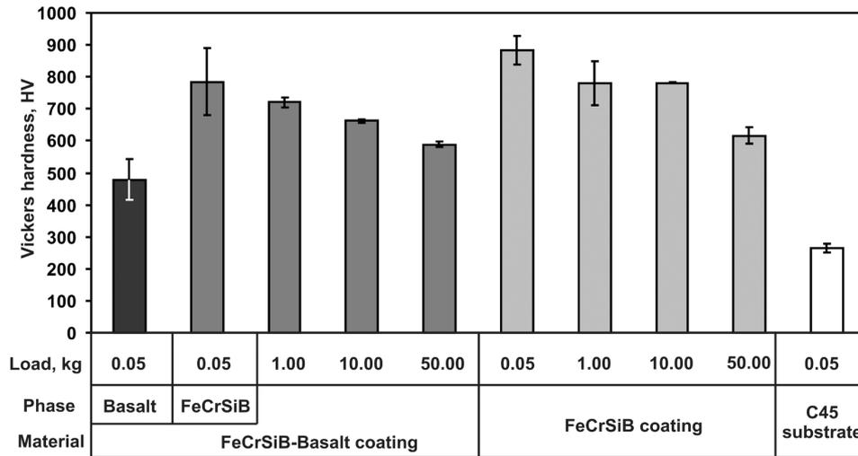
**Fig. 3.** Vickers hardness of HVOF sprayed coatings, basalt, steel phases and substrate measured after coating application.
