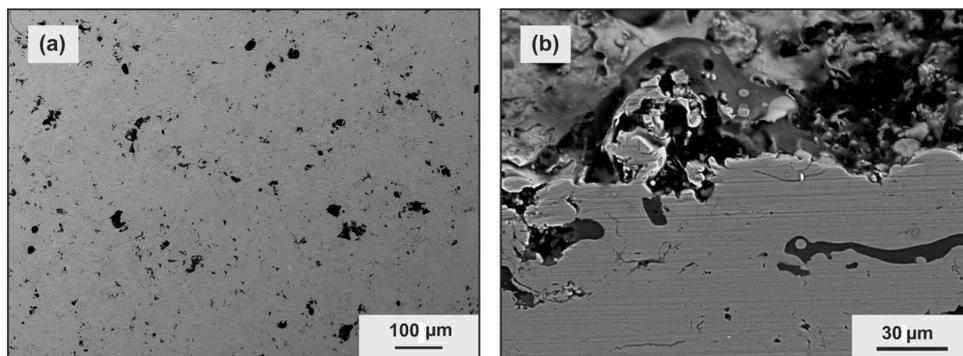
**Fig. 2.** SEM images of FeCrSiB-Basalt HVOF sprayed coating: (a) top view of the polished coating; (b) cross-section (top surface is not polished); dark areas indicate basalt.
