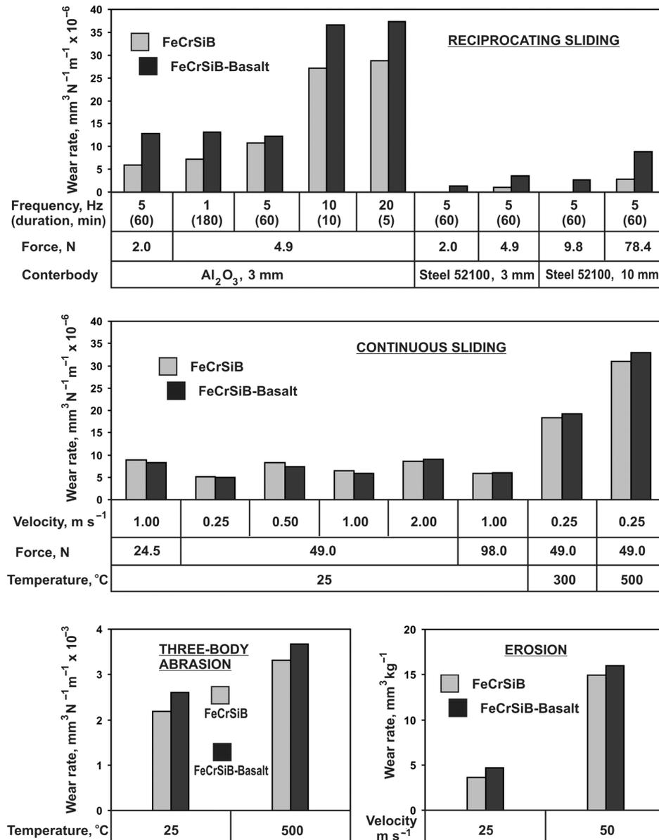
Fig. 4. Wear rates of coatings in various conditions.
