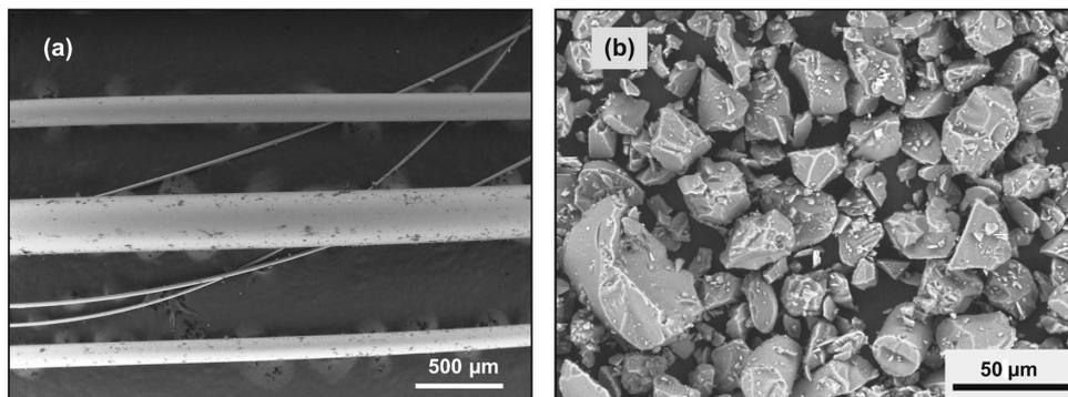
**Fig. 1.** SEM images: (a) original as-received basalt waste fibres of various thickness; (b) basalt powder after disintegrator milling.
