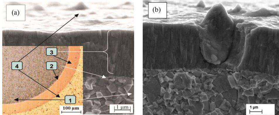
**Fig. 1.** (a) SEM image of the fractured surface of a TiN coating: (a) 1 – substrate; 2 – Ti adhesion layer; 3 – TiN layer; 4 – coating surface with macro-droplets; (b) cross-section of the coating with macro-droplets.
