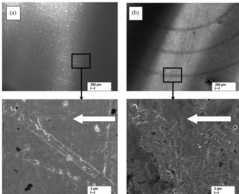
Fig. 5. SEM images of wear tracks of TiN after post-treatment: (a)  $R_a$  0.05; (b)  $R_a$  0.20 (arrow shows sliding direction).
