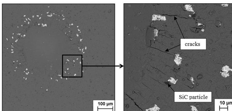
Fig. 2. SEM images of indents of adhesion test of coating (pre-treated 0.2 MPa).
