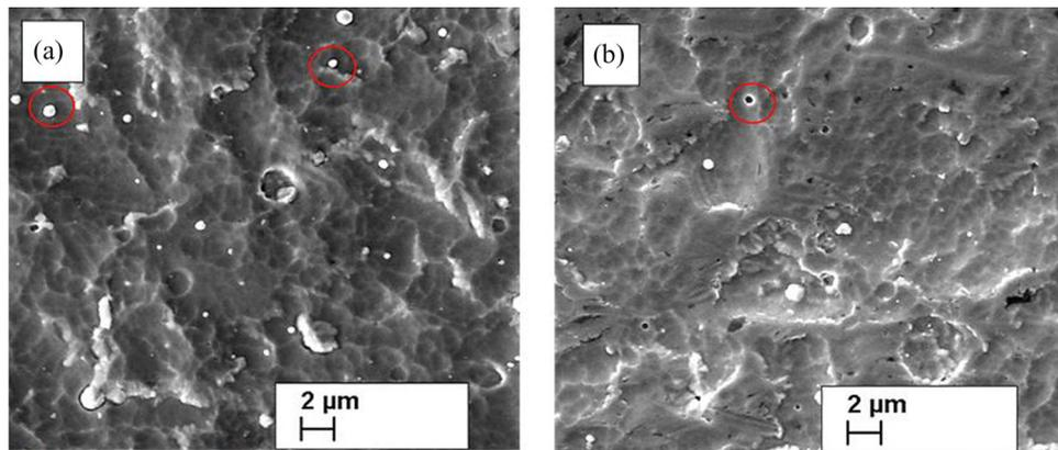
Fig. 4. SEM images of TiN coating surfaces: (a) as deposited; (b) post-treated.
