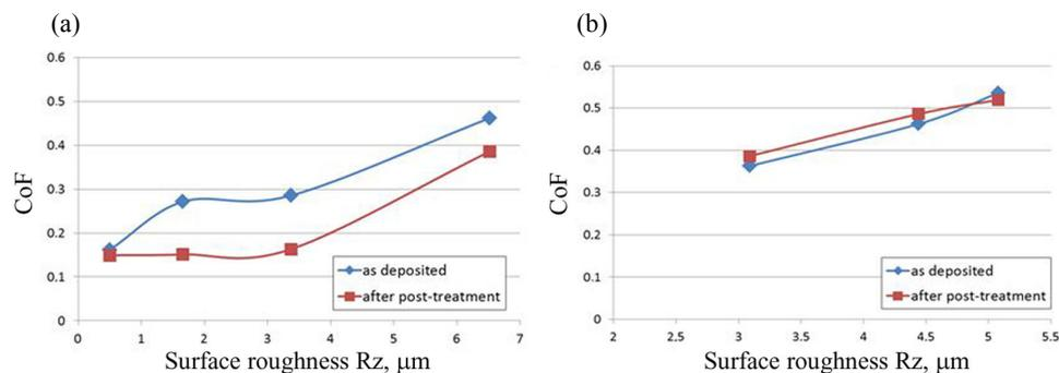
**Fig. 3.** The influence of the post-treatment of the TiN coating on the CoF: (a) grinded surface; (b) micro-blasted surface.
