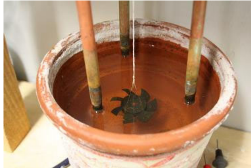
Fig. 22. Fan, lowered into the salt solution.
